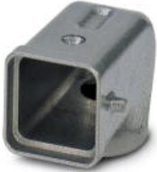
Sleeve housing, for single locking latch, height 48 mm, without screw connection, 1 x Pg11, lateral cable outlet, zinc die-cast
