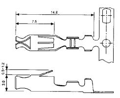
Part Number: 170219-1 and 170219-2 (Low mating force) Application Spec: 114-5016 Product Specifications:108-5012 Mates with 1.57 diameter pin
