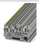
Sensor/actuator terminal block, Connection method: Spring-cage connection, Cross section: 0.08 mm² - 4 mm², AWG: 28 - 12, Width: 5.2 mm, Color: gray, Mounting type: NS 35/7,5, NS 35/15
