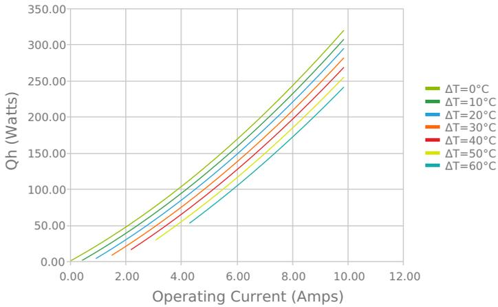
Total Heat Dissipated at Hot Side (Qh=Qc+Pin)
