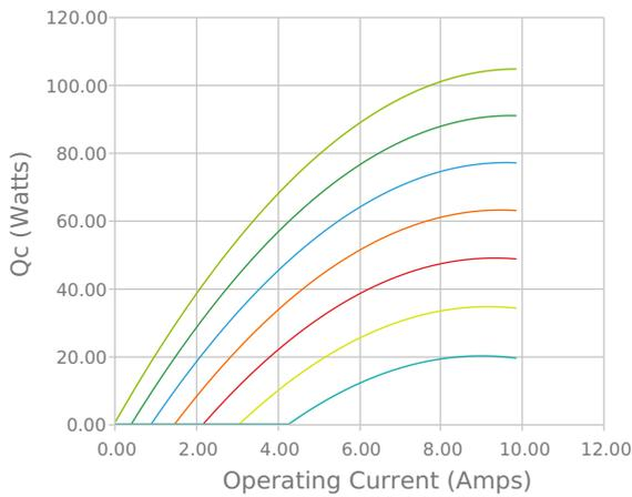
Heat Pumped at Cold Side
