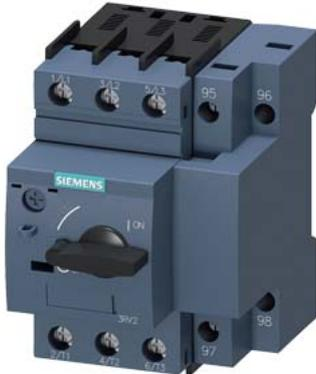
Circuit breaker size S00 for motor protection, CLASS 10 with overload relay function A-release 0.55...0.8 A N-release 10 A screw terminal Standard switching capacity
