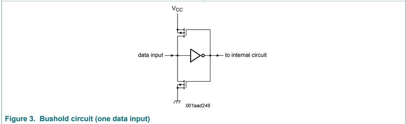
Figure 3. Bushold circuit (one data input)
