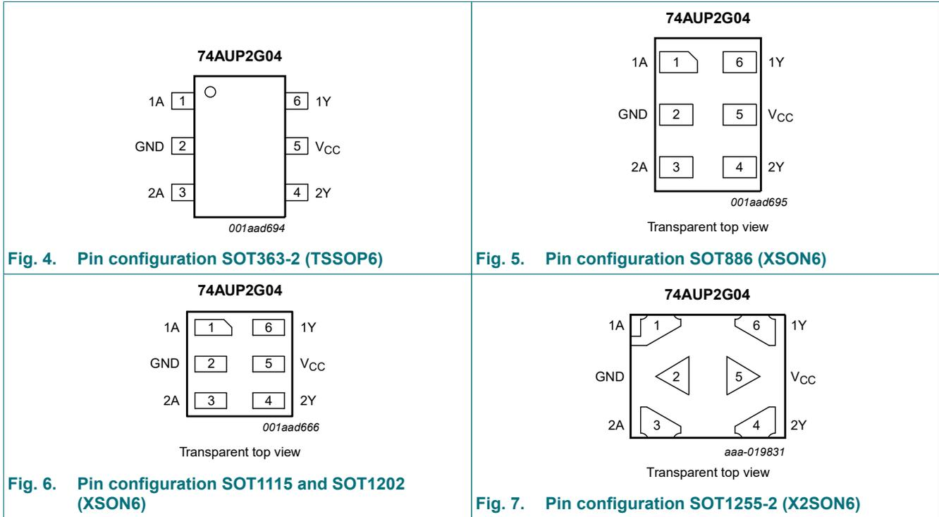
Fig. 4. Pin configuration SOT363-2 (TSSOP6)
