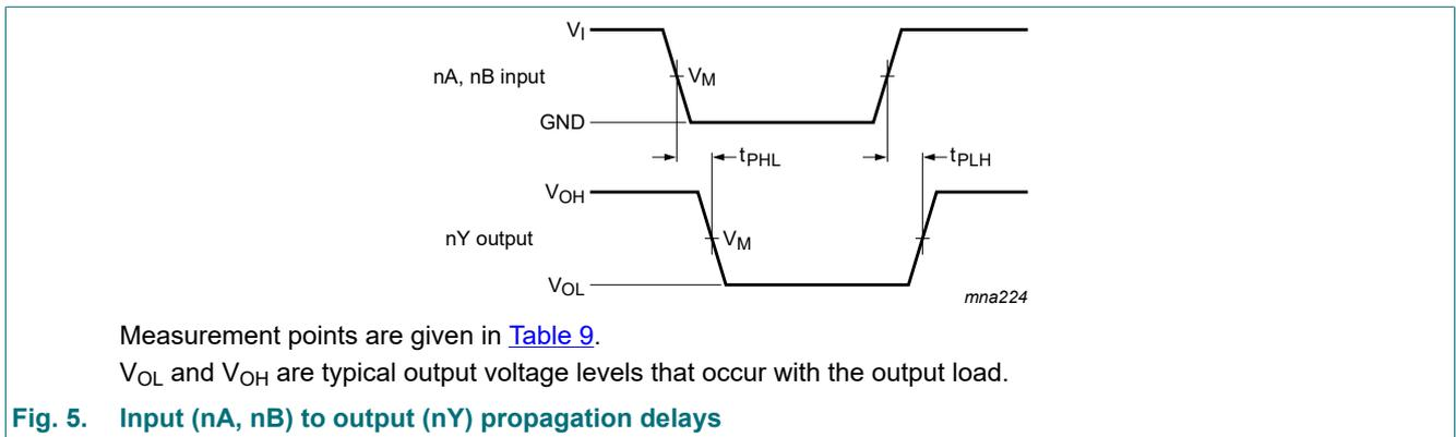
**Fig. 5. Input (nA, nB) to output (nY) propagation delays**
