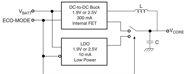
Low undershoot voltage is expected when going from PWM to LDO mode and vice-versa. The circuit is designed in order to avoid any spikes when transition between two modes is enabled.
