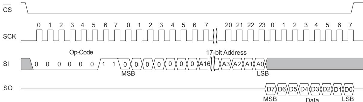
Figure 11. Burst Mode Read Instruction Timing
