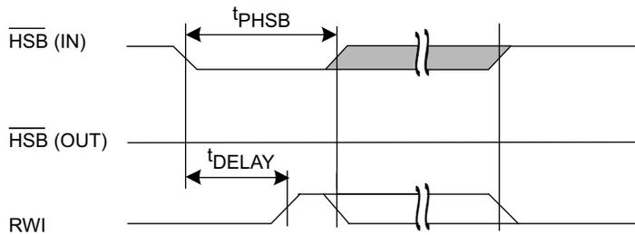
HSB pin is driven HIGH to V<sub>CC</sub> only by Internal 100 KΩ resistor, HSB driver is disabled
