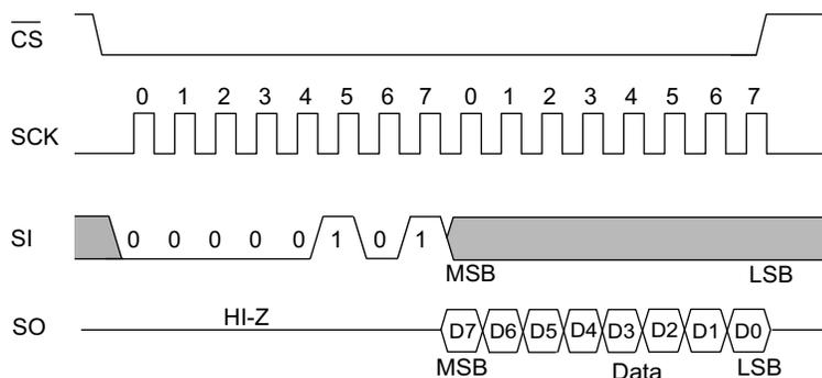
Figure 7. Write Status Register (WRSR) Instruction Timing
