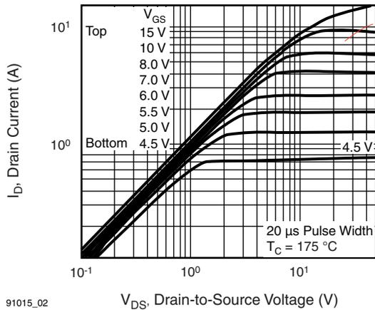
**Fig. 2 - Typical Output Characteristics,  $T_C = 175^\circ\text{C}$**
