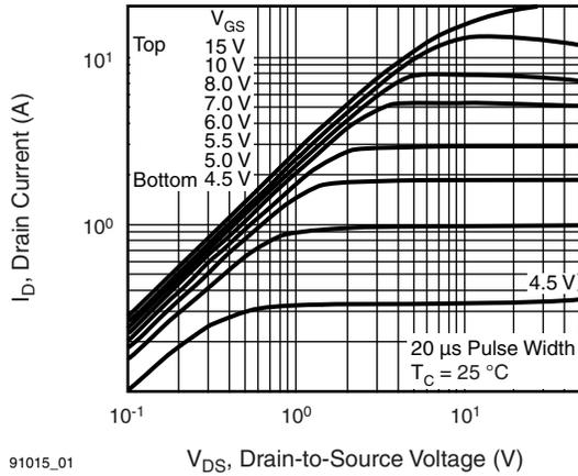
**Fig. 1 - Typical Output Characteristics,  $T_C = 25^\circ\text{C}$**
