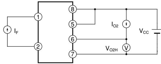
**Fig.3 Test Circuit for O<sub>2</sub> Low Level Output Voltage**
