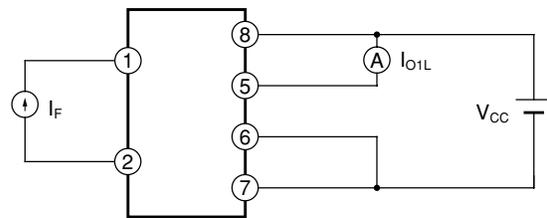
**Fig.5 Test Circuit for O<sub>2</sub> Leak Current**
