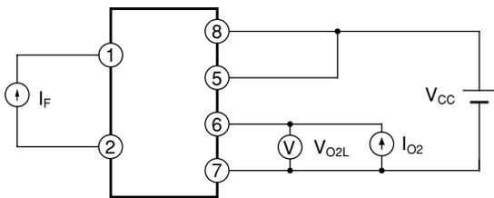
**Fig.4 Test Circuit for O<sub>1</sub> Leak Current**
