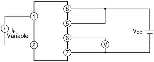
**Fig.8 Test Circuit for Response Time**
