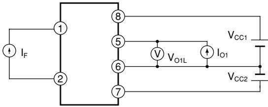
**Fig.2 Test Circuit for O<sub>2</sub> High Level Output Voltage**
