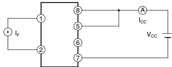
**Fig.7 Test Circuit for "Low→High" Input Threshold Current**
