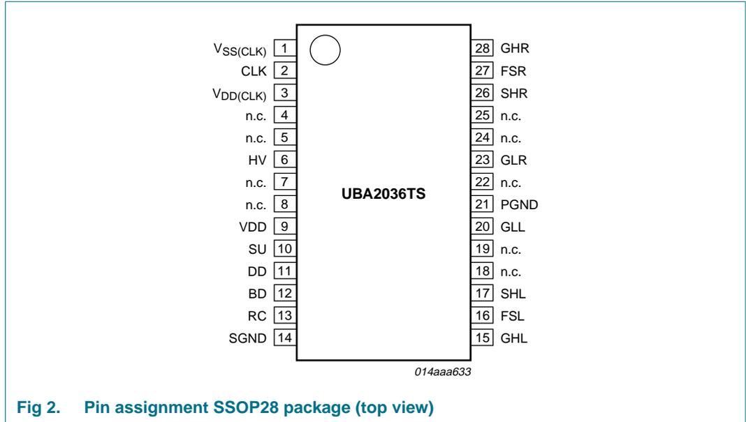
Fig 2. Pin assignment SSOP28 package (top view)
