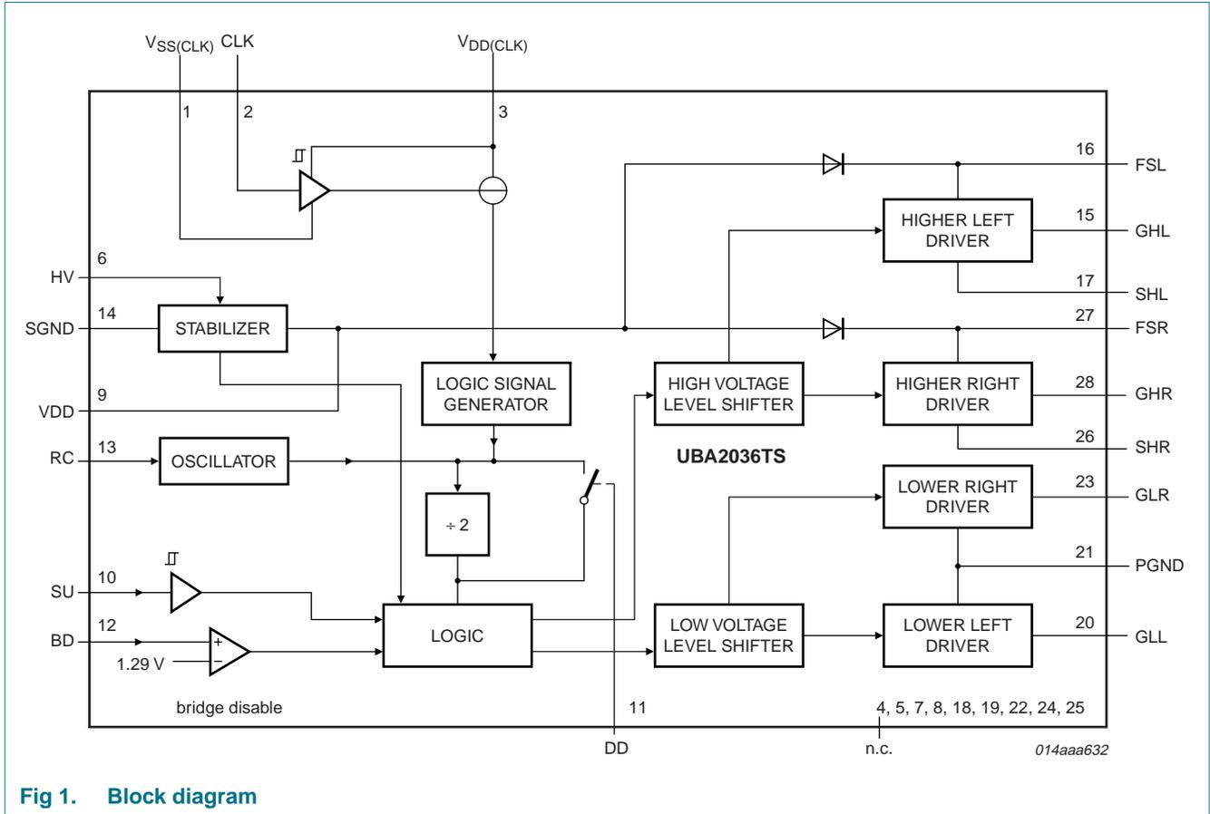
**Fig 1. Block diagram**
