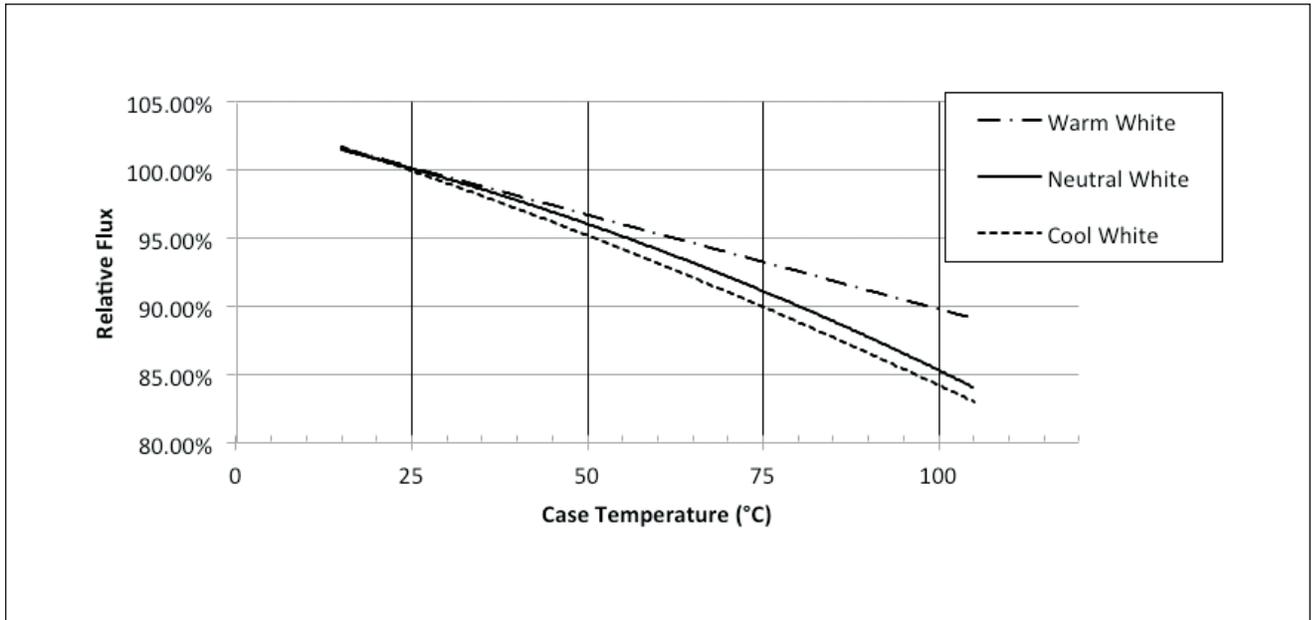
**Figure 4: Typical DC ccy Shift vs. Case Temperature**
