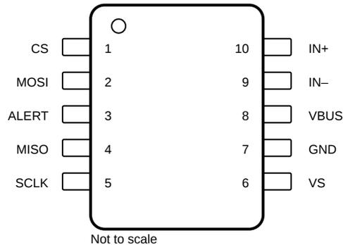
**Figure 5-1. DGS Package 10-Pin VSSOP Top View**
