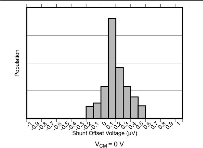
Figure 6-3. Shunt Input Offset Voltage Production Distribution
