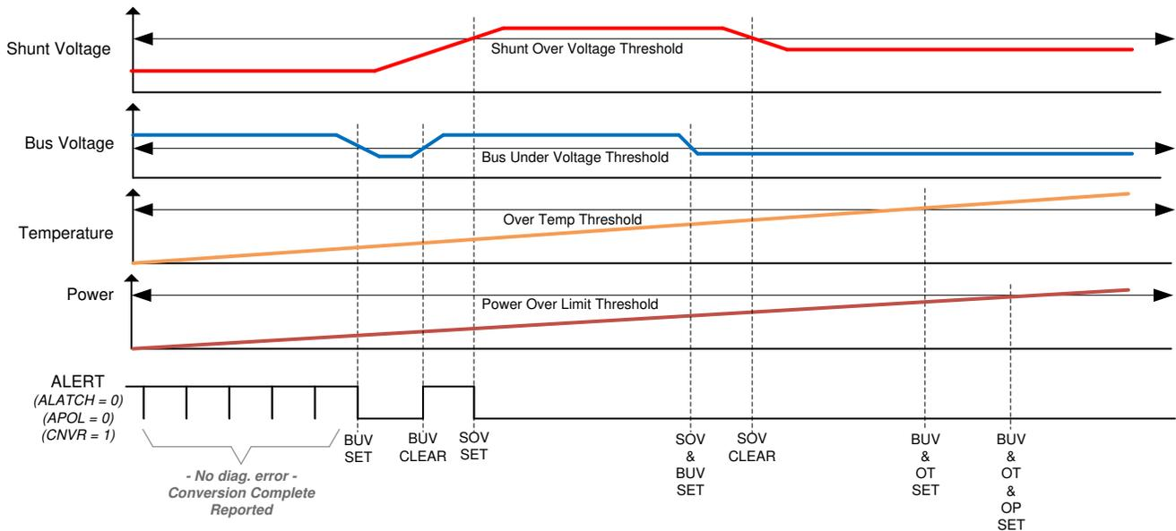
**Figure 7-6. Multi-Alert Configuration**
