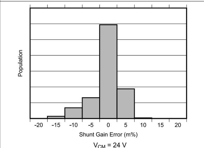
Figure 6-7. Shunt Input Gain Error Production Distribution
