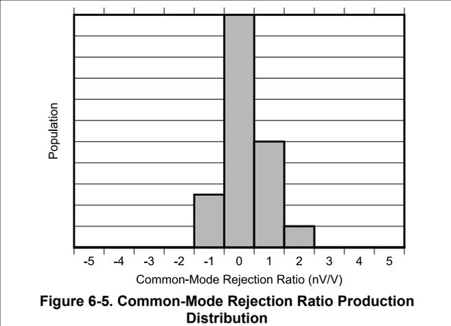
Figure 6-5. Common-Mode Rejection Ratio Production Distribution
