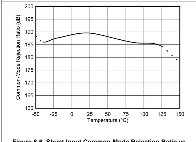
Figure 6-6. Shunt Input Common-Mode Rejection Ratio vs. Temperature
