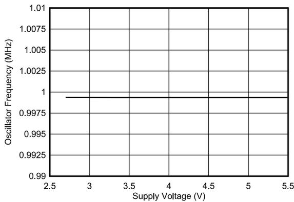
Figure 6-24. Internal Clock Frequency vs. Power Supply
