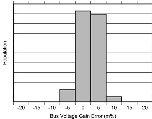
Figure 6-12. Bus Input Gain Error Production Distribution
