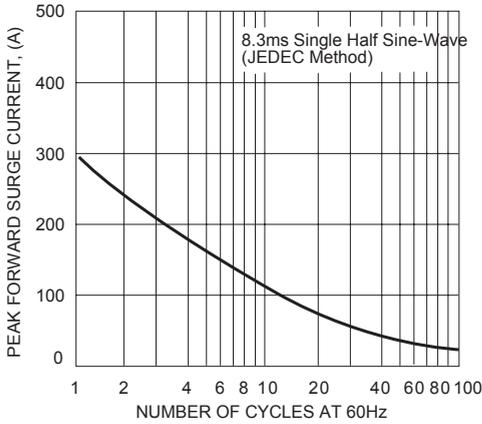
FIG. 2 - TYPICAL FORWARD CURRENT DERATING CURVE
