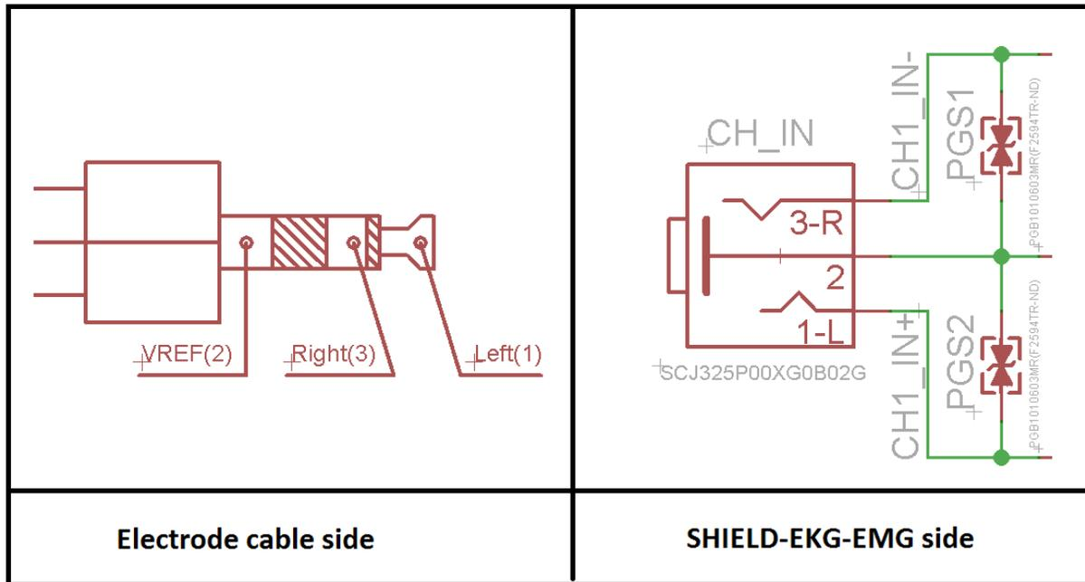
Note that connecting active electrode that way will probably lead to electrical shock for SHIELD-EKG-EMG. Only passive electrodes can be used with SHIELD-EKG-EMG.
