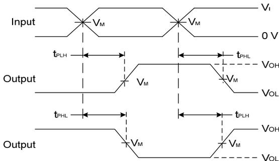
**Voltage Waveform Propagation Delay Times
