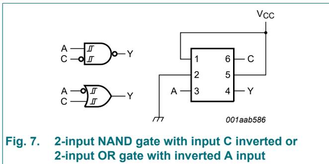
Fig. 7. 2-input NAND gate with input C inverted or 2-input OR gate with inverted A input
