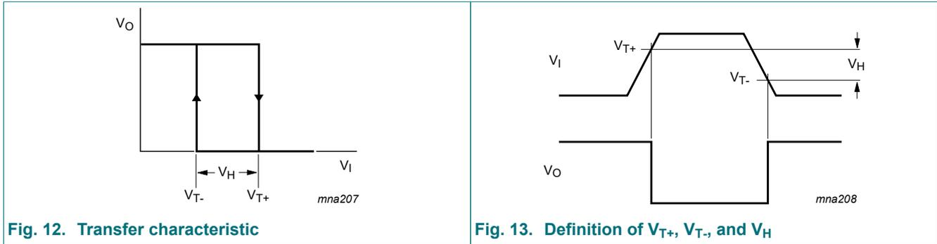
Fig. 12. Transfer characteristic
