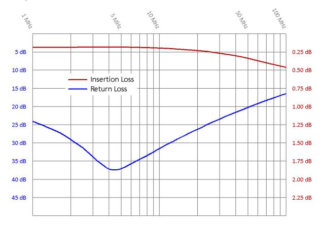
Figure 5. Typical frequency response for EN-85e.
