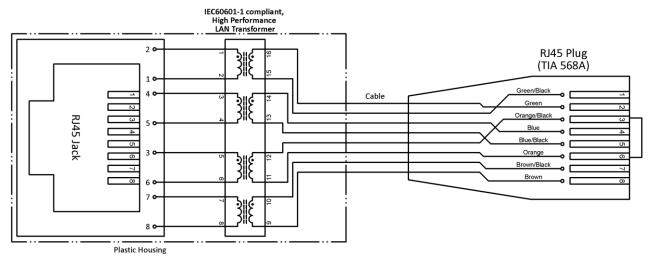
Figure 6. Schematic diagram of the EN-85e.
