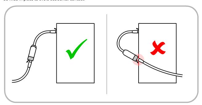
Figure 3. Positioning of EN-85e when connecting to PCs or other Ethernet-capable devices with metallic surfaces.
