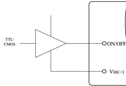
Figure 11. Direct Logic Drive
