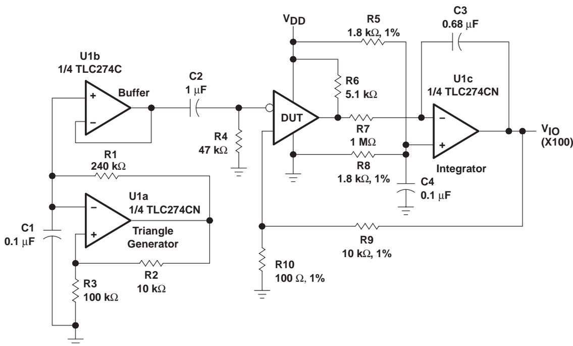
**Figure 2. Circuit for Input Offset Voltage Measurement**
