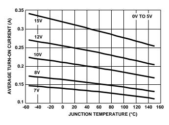
FIGURE 10. GATE DRIVER AVERAGE TURN-ON CURRENT
