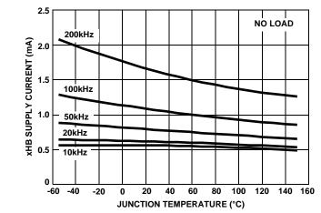
FIGURE 6. FLOATING SUPPLY SWITCHING BIAS CURRENT
