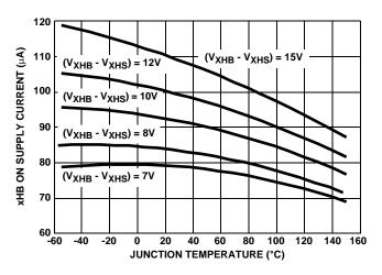
FIGURE 4. FLOATING SUPPLY ON BIAS CURRENT
