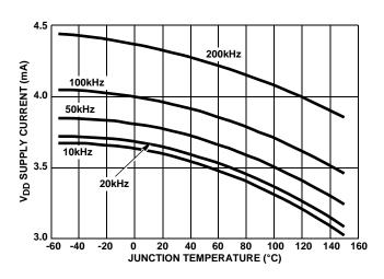
FIGURE 2. VDD SUPPLY CURRENT vs SWITCHING FREQUENCY
