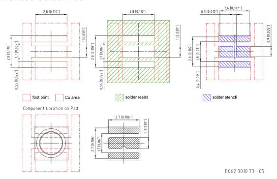
For superior solder joint connectivity results we recommend soldering under standard nitrogen atmosphere. Package not suitable for any kind of wet cleaning or ultrasonic cleaning.
