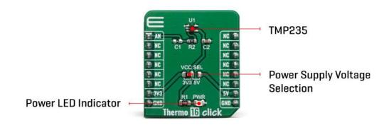
The TMP23X devices are a family of precision CMOS integrated-circuit linear analog temperature sensors with an output voltage proportional to temperature engineers can use in multiple analog temperature sensing applications. The TMP235 temperature sensor have an accuracy from 0°C to 70°C of ±1.25°C and provides a positive slope output of 10 mV/°C over the full –40°C to +150°C temperature range.
