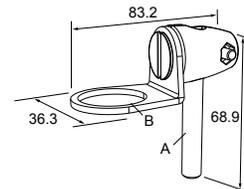
**Bolt thread:** SMB30FA, A= 3/8 - 16 x 2 in; SMB30FAM10, A= M10 - 1.5 x 50
