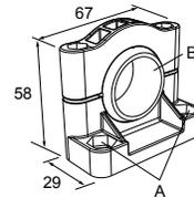
**Hole center spacing:** A=ø 50.8
