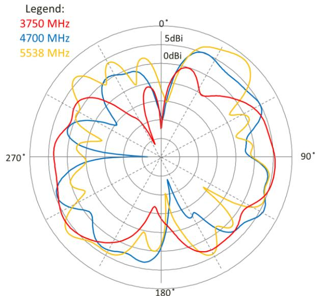
Data measured in free space with hinge at 90 degree bend
