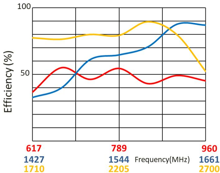
Data measured in free space with hinge at 90 degree bend
