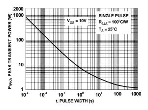
Figure 10. Single Pulse Maximum Power Dissipation
