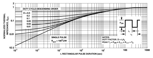
Figure 11. Transient Thermal Response Curve
