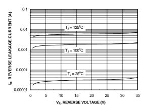
Figure 24. SyncFET body diode reverses leakage versus drain-source voltage and temperature
