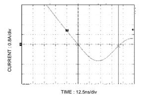
Figure 23. Non-SyncFET (FDZ4670) body diode reverse recovery characteristic
