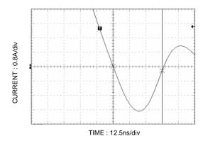
Figure 22. FDZ4670S SyncFET body diode reverse recovery characteristic
