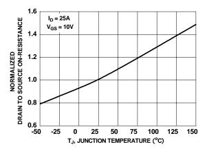
Figure 3. Normalized On-Resistance vs Junction Temperature
