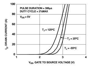
Figure 5. Transfer Characteristics
