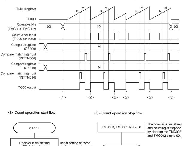
Figure 6-32. Example of Software Processing in Clear & Start Mode Entered by TI000 Pin Valid Edge Input
