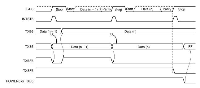
Figure 14-20. Timing of Ending Continuous Transmission
