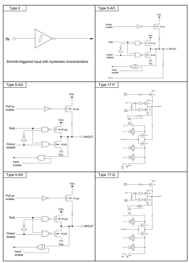
Figure 2-1. Pin I/O Circuit List (2/2)
