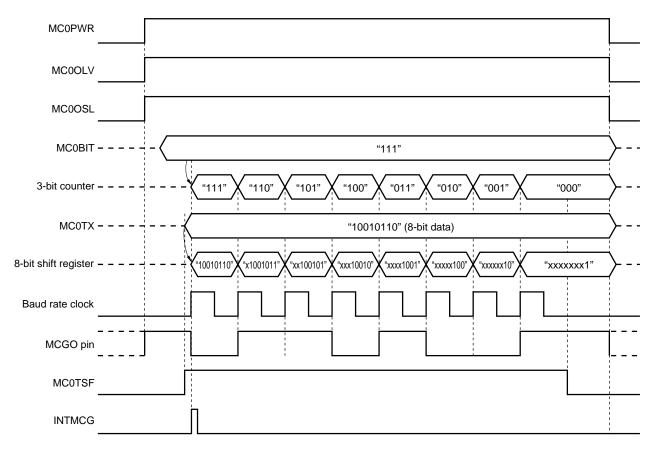
Figure 16-9. Timing of Bit Sequential Buffer Mode (LSB First) (2/4)
