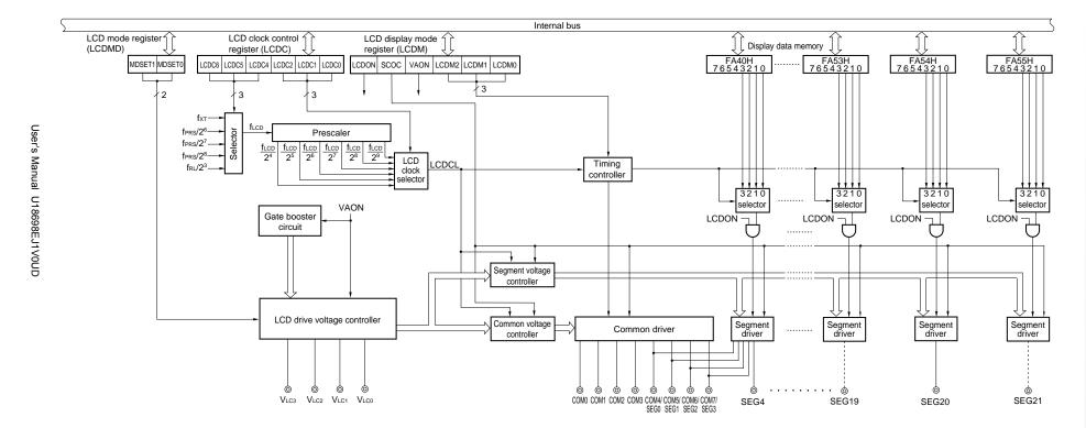
Figure 15-1. Block Diagram of LCD Controller/Driver
