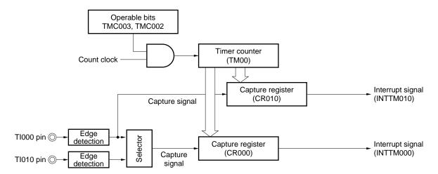
**Remark** If both CR000 and CR010 are used as capture registers in the free-running timer mode, the TO00 output level is not inverted.
