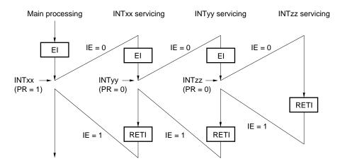
During servicing of interrupt INTxx, two interrupt requests, INTyy and INTzz, are acknowledged, and multiple interrupt servicing takes place. Before each interrupt request is acknowledged, the EI instruction must always be issued to enable interrupt request acknowledgment.
