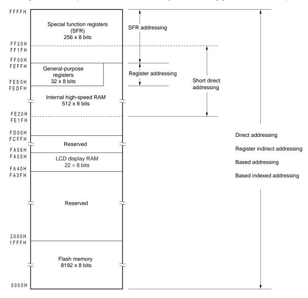
Figure 3-5. Correspondence Between Data Memory and Addressing (µPD78F0400, 78F0410)
