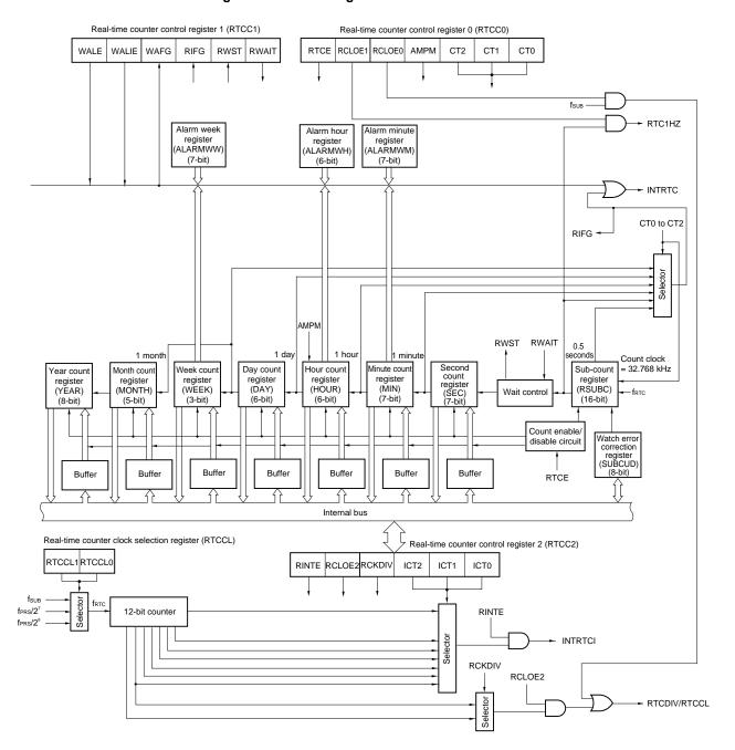
Figure 9-1. Block Diagram of Real-Time Counter
