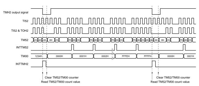
Figure 6-55. Operation Timing of External 24-bit Event Counter
