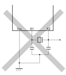
**Remark** When using the subsystem clock, replace X1 and X2 with XT1 and XT2, respectively. Also, insert resistors in series on the XT2 side.
