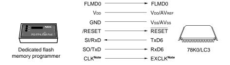
**Note** The above figure illustrates an example of wiring when using the clock output from the PG-FP4 or FL-PR4. When using the clock output from the PG-FPL3 or FP-LITE3, connect CLK to X1/P121, and connect its inverted signal to X2/EXCLK/P122.
