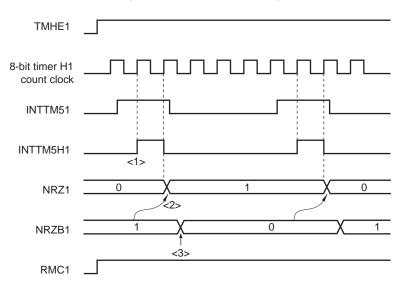
Figure 8-15. Transfer Timing
