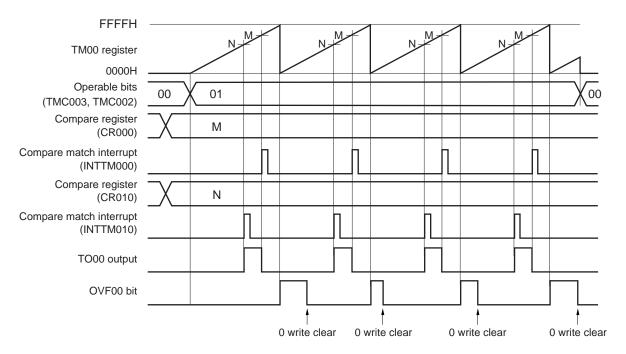
This is an application example where two compare registers are used in the free-running timer mode. The TO00 output level is reversed each time the count value of TM00 matches the set value of CR000 or CR010. When the count value matches the register value, the INTTM000 or INTTM010 signal is generated.
