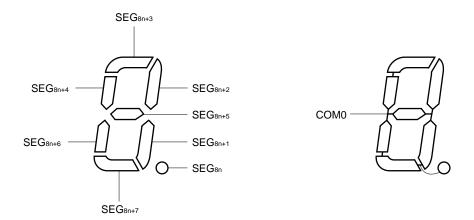
Figure 15-10. Static LCD Display Pattern and Electrode Connections
