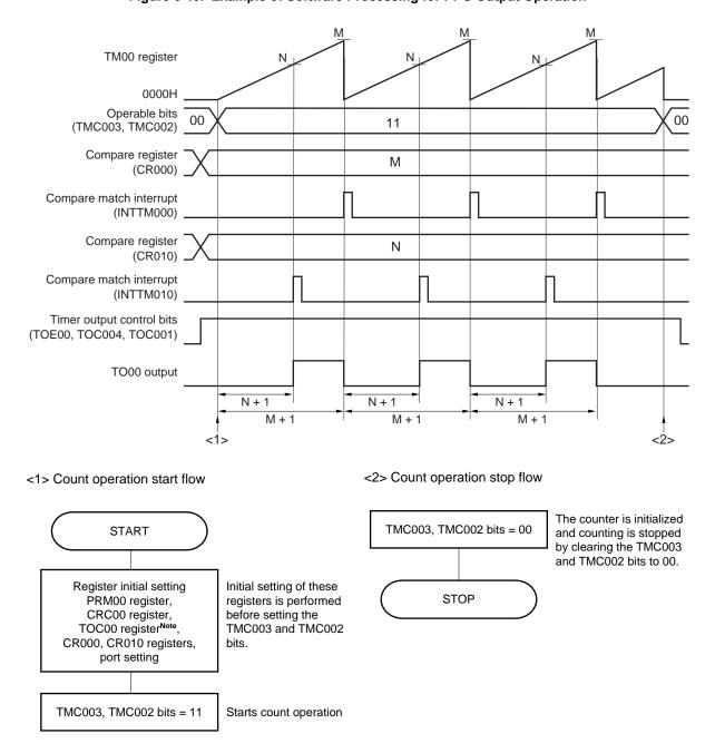
Figure 6-43. Example of Software Processing for PPG Output Operation
