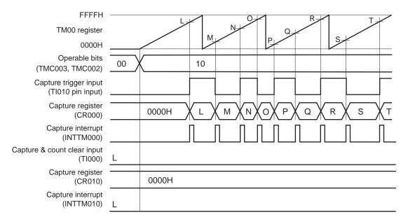
This is a timing example where an edge is not input to the TI000 pin, in an application where the count value is captured to CR000 when the rising or falling edge of the TI010 pin is detected.
