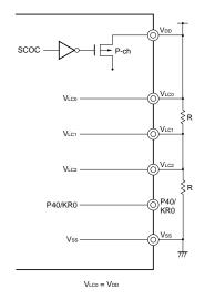
(d) 1/2 bias method (MDSET1, MDSET0 = 0, 0) (example of VDD = 5 V, VLC0 = 3 V)
