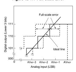
Figure 12-19. Differential Linearity Error
