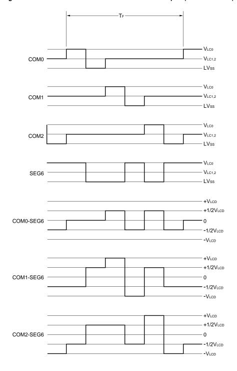
Figure 15-18. Three-Time-Slice LCD Drive Waveform Examples (1/2 Bias Method)
