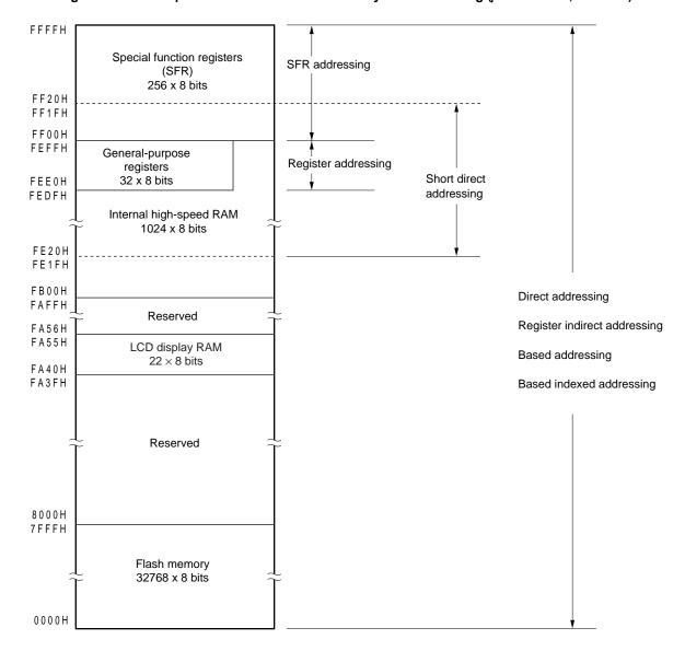
Figure 3-8. Correspondence Between Data Memory and Addressing (μPD78F0403, 78F0413)
