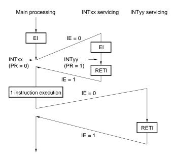
Interrupt request INTyy issued during servicing of interrupt INTxx is not acknowledged because its priority is lower than that of INTxx, and multiple interrupt servicing does not take place. The INTyy interrupt request is held pending, and is acknowledged following execution of one main processing instruction.
