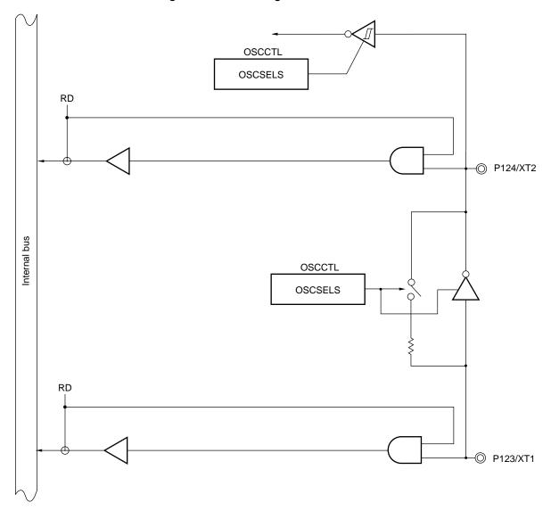
Figure 4-13. Block Diagram of P123 and P124
