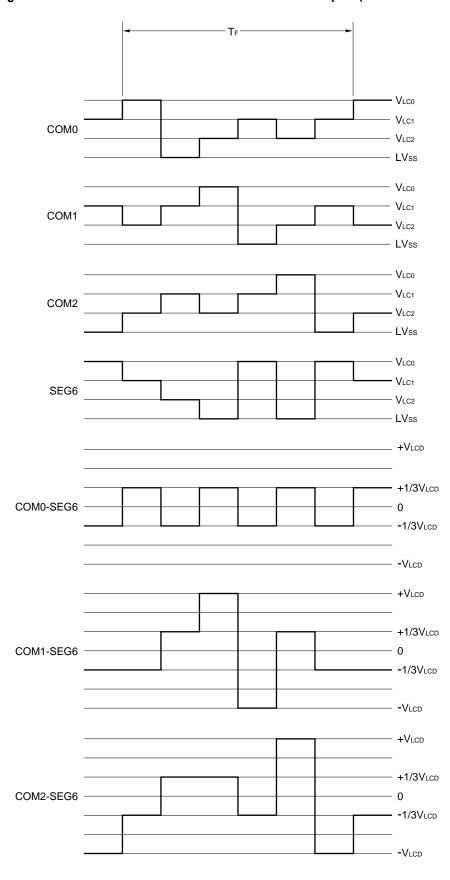
Figure 15-19. Three-Time-Slice LCD Drive Waveform Examples (1/3 Bias Method)
