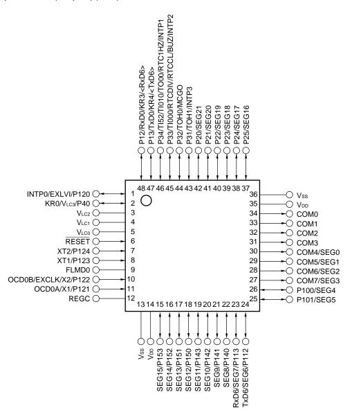
Cautions 1. Connect the REGC pin to Vss via a capacitor (0.47 to 1  $\mu$ F: recommended).
