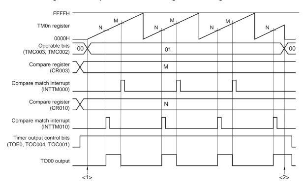
Figure 6-40. Example of Software Processing in Free-Running Timer Mode
