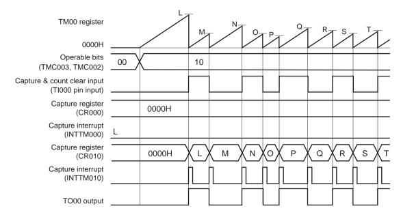
This is an application example where the count value is captured to CR010, TM00 is cleared, and the TO00 output is inverted when the rising or falling edge of the TI000 pin is detected.
