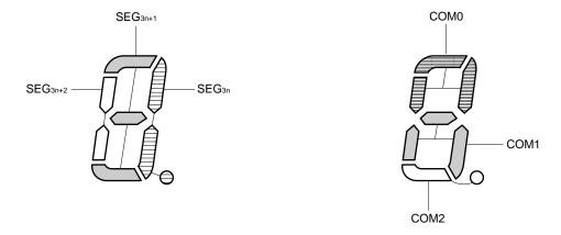
Figure 15-16. Three-Time-Slice LCD Display Pattern and Electrode Connections
