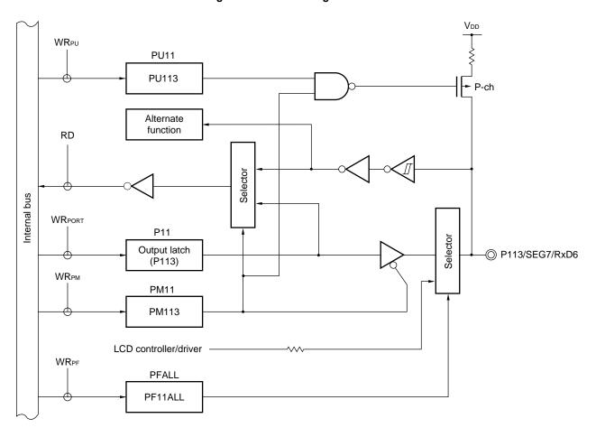
Figure 4-10. Block Diagram of P113
