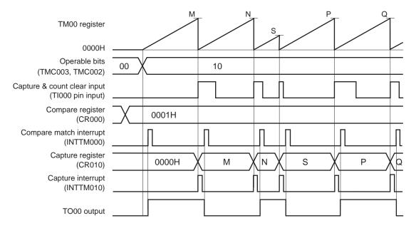
This is an application example where the TO00 output level is inverted when the count value has been captured & cleared.
