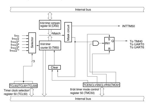
Figure 7-1. Block Diagram of 8-Bit Timer/Event Counter 50
