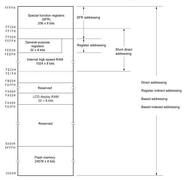
Figure 3-7. Correspondence Between Data Memory and Addressing (μPD78F0402, 78F0412)
