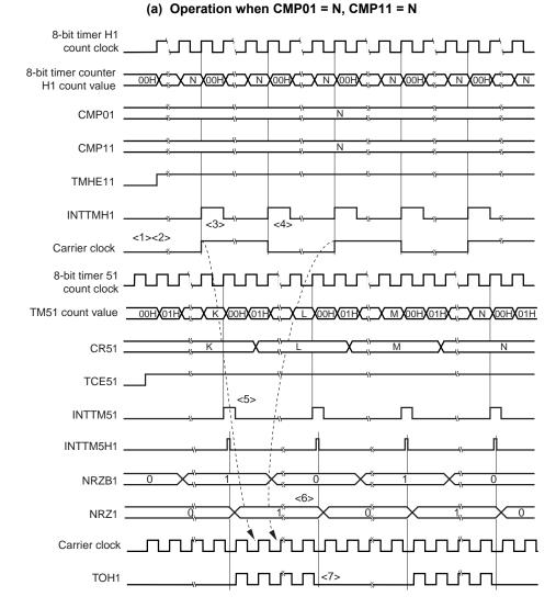
Figure 8-17. Carrier Generator Mode Operation Timing (1/3)
