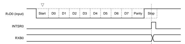
Figure 13-10. Reception Completion Interrupt Request Timing
