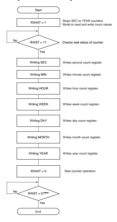
Figure 9-20. Procedure for Writing Real-Time Counter
