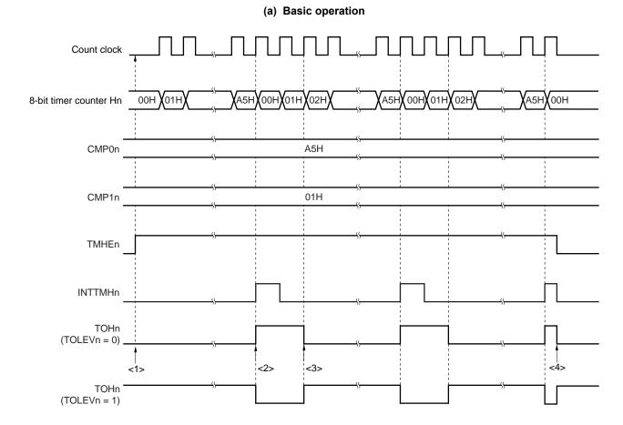
Figure 8-14. Operation Timing in PWM Output Mode (1/4)
