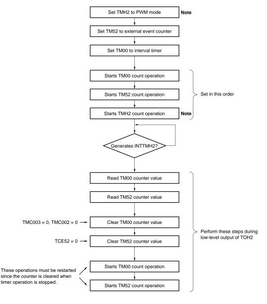
Figure 6-56. Operation Flowchart of External 24-bit Event Counter
