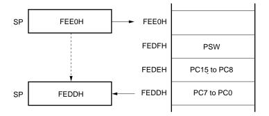
Figure 3-13. Data to Be Restored from Stack Memory
