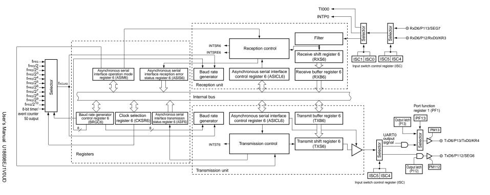
Figure 14-4. Block Diagram of Serial Interface UART6
