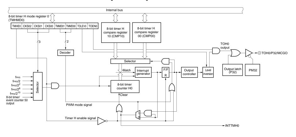
Figure 8-1. Block Diagram of 8-Bit Timer H0
