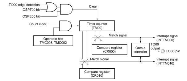
Figure 6-44. Block Diagram of One-Shot Pulse Output Operation
