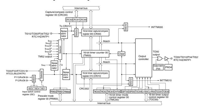
Cautions 1. The valid edge of Tl010 and timer output (TO00) cannot be used for the P34 pin at the same time. Select either of the functions.
