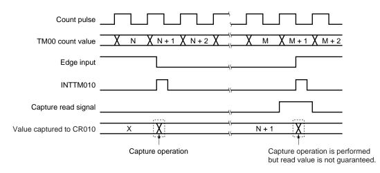
Figure 6-60. Timing of Holding Data by Capture Register
