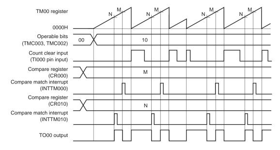
(a) and (b) differ as follows depending on the setting of bit 1 (TMC001) of the 16-bit timer mode control register 01 (TMC00).
