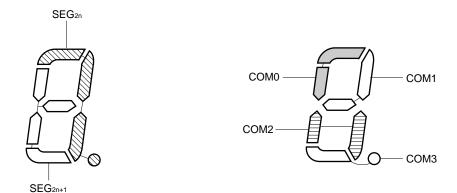
Figure 15-20. Four-Time-Slice LCD Display Pattern and Electrode Connections
