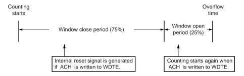
Caution The first writing to WDTE after a reset release clears the watchdog timer, if it is made before the overflow time regardless of the timing of the writing, and the watchdog timer starts counting again.
