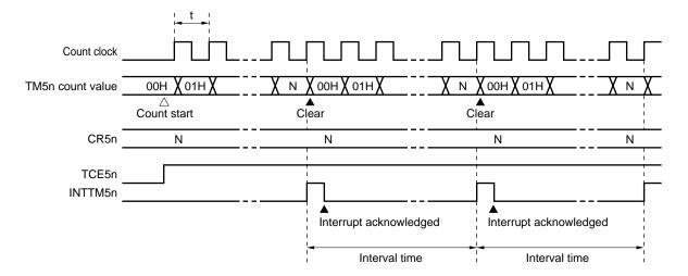
Remark Interval time =  $(N + 1) \times t$  N = 01H to FFHn = 0 to 2
