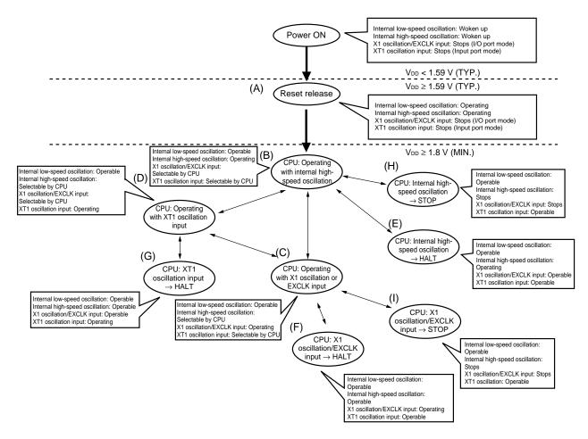
**Remark** In the 2.7 V/1.59 V POC mode (option byte: POCMODE = 1), the CPU clock status changes to (A) in the above figure when the supply voltage exceeds 2.7 V (TYP.), and to (B) after reset processing (11 to 47  $\mu$ s (TYP.)).
