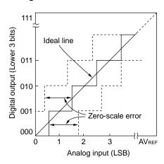
Figure 12-18. Integral Linearity Error
