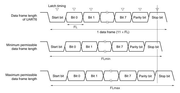
Figure 14-27. Permissible Baud Rate Range During Reception
