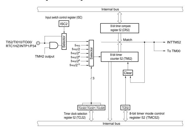
Figure 7-3. Block Diagram of 8-Bit Timer/Event Counter 52
