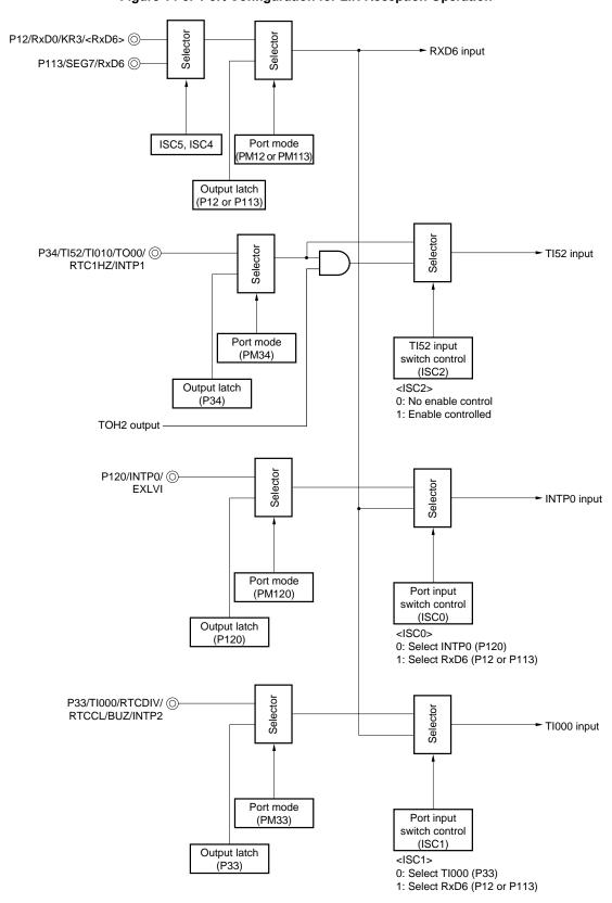
Figure 14-3. Port Configuration for LIN Reception Operation
