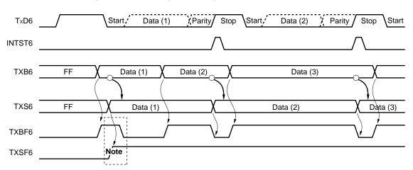
Figure 14-19. Timing of Starting Continuous Transmission
