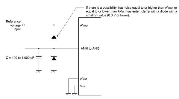
Figure 12-20. Analog Input Pin Connection
