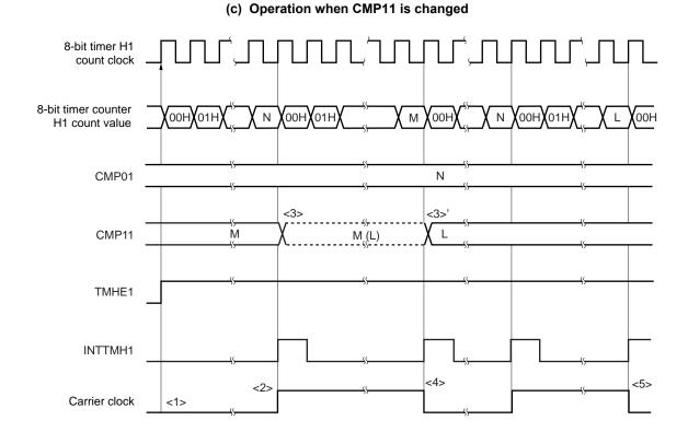
Figure 8-17. Carrier Generator Mode Operation Timing (3/3)
