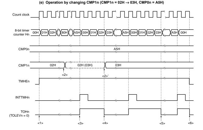
Figure 8-14. Operation Timing in PWM Output Mode (4/4)
