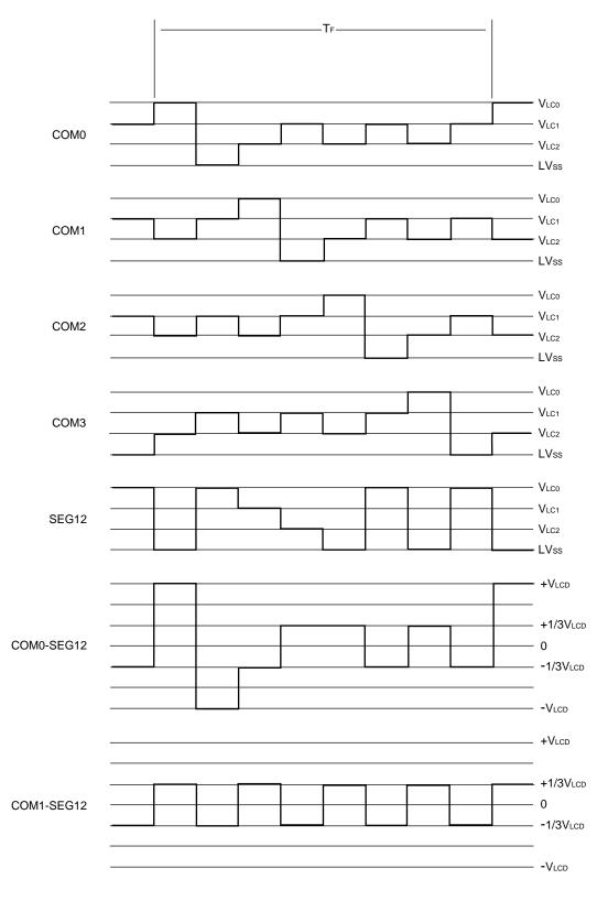
Figure 15-22. Four-Time-Slice LCD Drive Waveform Examples (1/3 Bias Method)
