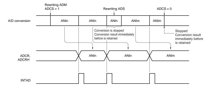
Figure 12-13. A/D Conversion Operation
