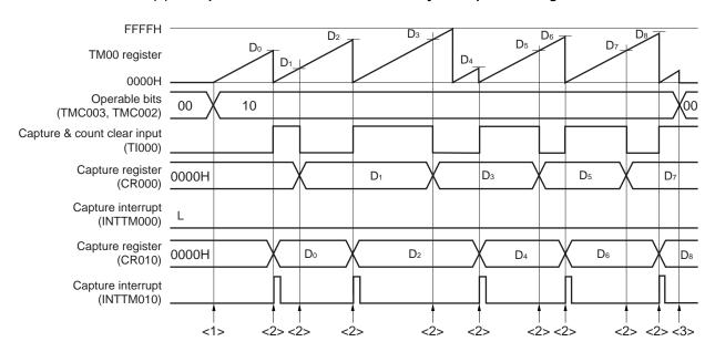
Figure 6-53. Example of Software Processing for Pulse Width Measurement (2/2)
