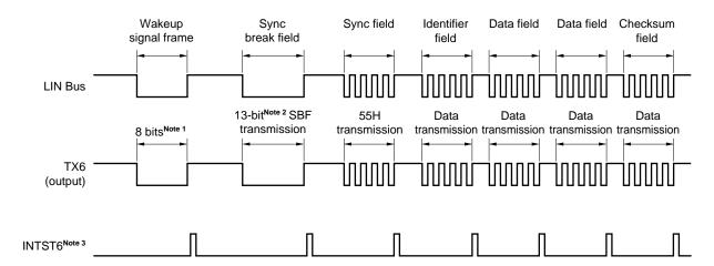
Figure 14-1. LIN Transmission Operation
