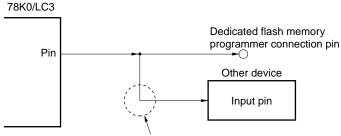
If the signal output by the 78K0/LC3 in the flash memory programming mode affects the other device, isolate the signal of the other device.
