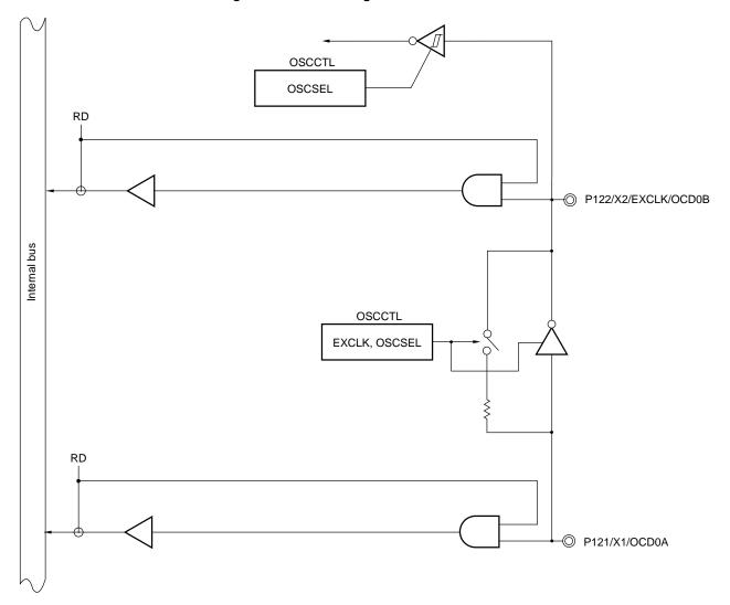
Figure 4-12. Block Diagram of P121 and P122
