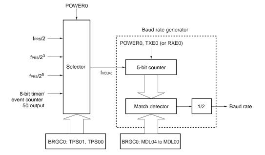
Figure 13-12. Configuration of Baud Rate Generator
