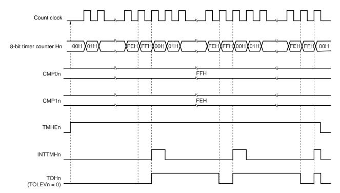
Figure 8-14. Operation Timing in PWM Output Mode (3/4)
