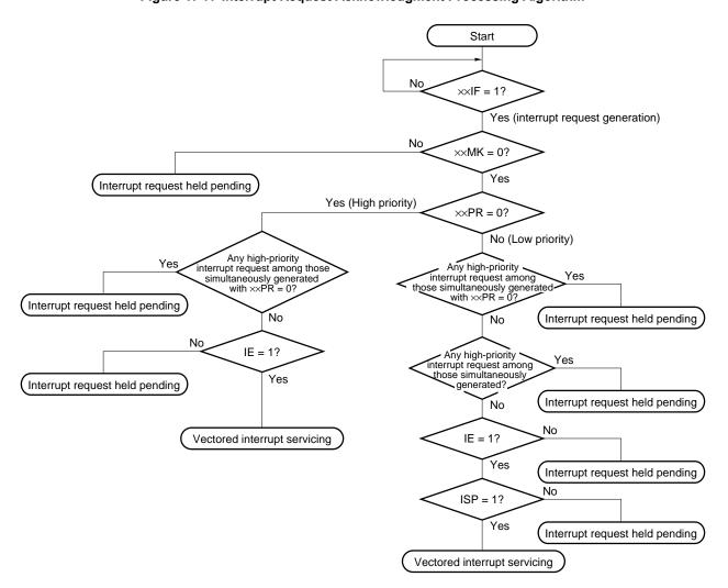
Figure 17-7. Interrupt Request Acknowledgment Processing Algorithm
