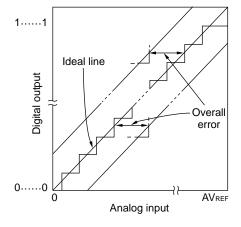
Figure 12-15. Quantization Error
