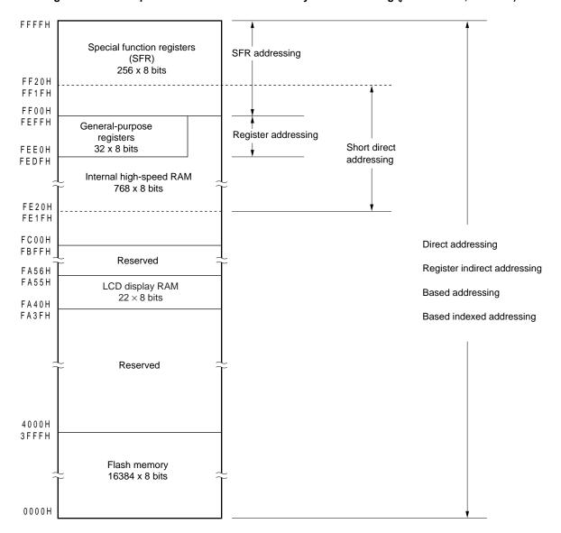
Figure 3-6. Correspondence Between Data Memory and Addressing (μPD78F0401, 78F0411)
