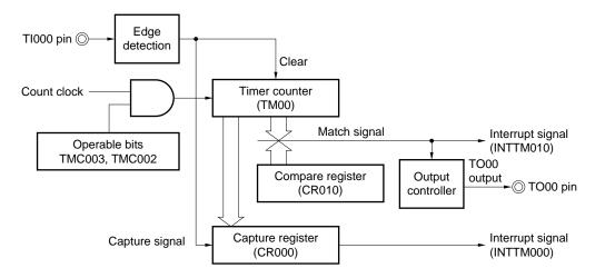
Figure 6-28. Timing Example of Clear & Start Mode Entered by Tl000 Pin Valid Edge Input (CR000: Capture Register, CR010: Compare Register) (1/2)
