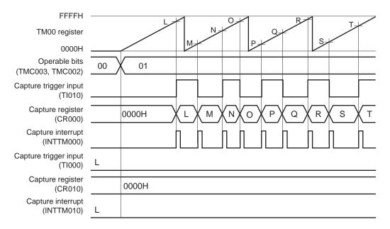
This is an application example where both the edges of the TI010 pin are detected and the count value is captured to CR000 in the free-running timer mode.
