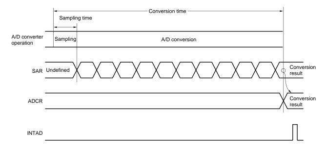
Figure 12-11. Basic Operation of A/D Converter
