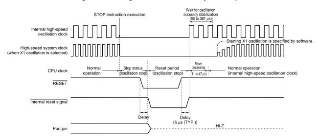
Figure 20-4. Timing of Reset in STOP Mode by RESET Input
