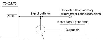
In the flash memory programming mode, the signal output by the reset signal generator collides with the signal output by the dedicated flash memory programmer. Therefore, isolate the signal of the reset signal generator.
