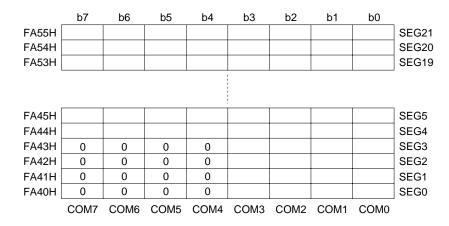
Caution No memory is allocated to the higher 4 bits of FA40H to FA43H. Be sure to set there bits to 0.
