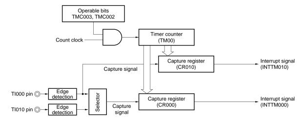
Figure 6-48. Block Diagram of Pulse Width Measurement (Clear & Start Mode Entered by Tl000 Pin Valid Edge Input)
