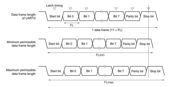
Figure 13-13. Permissible Baud Rate Range During Reception
