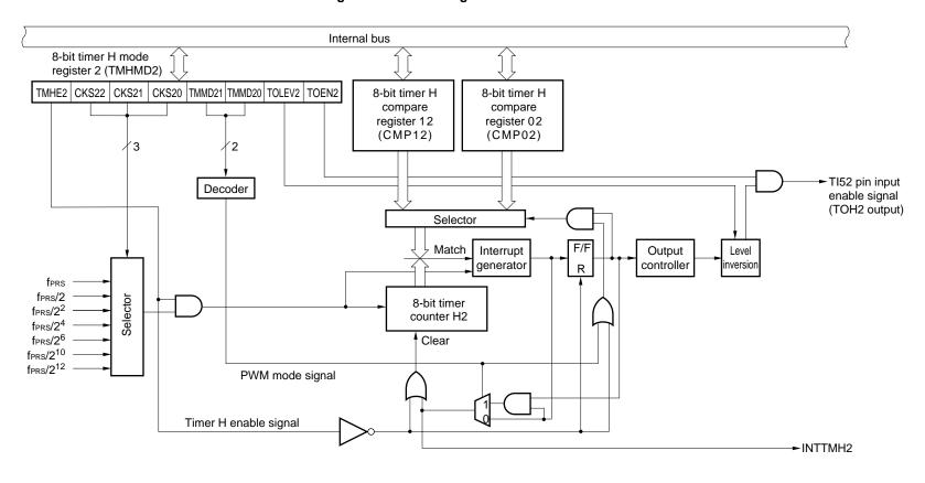
Figure 8-3. Block Diagram of 8-Bit Timer H2
