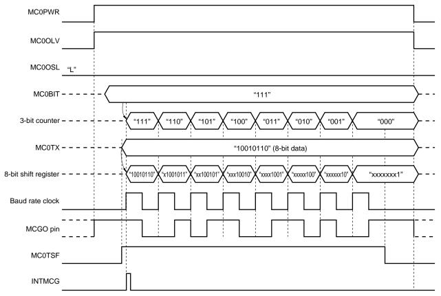
Figure 16-8. Timing of Manchester Code Generator Mode (LSB First) (2/4)
