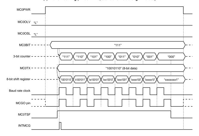
Figure 16-8. Timing of Manchester Code Generator Mode (LSB First) (3/4)
