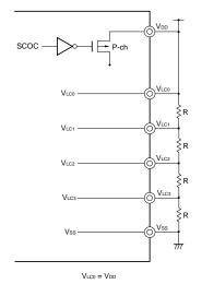
(f) 1/3 bias method (MDSET1, MDSET0 = 0, 0) (example of V<sub>DD</sub> = 5 V, V<sub>LC0</sub> = 3 V)
