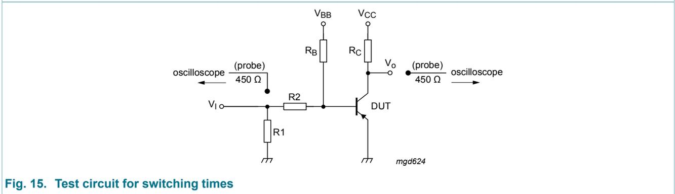
Fig. 15. Test circuit for switching times
