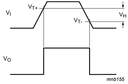
$V_{T+}$  and  $V_{T-}$  limits are at 70 % and 20 %.
