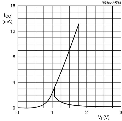
Fig. 16. Typical 74LVC1G57-Q100 transfer characteristic;  $V_{CC} = 3.0$  V
