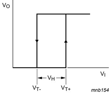
Fig. 14. Transfer characteristic
