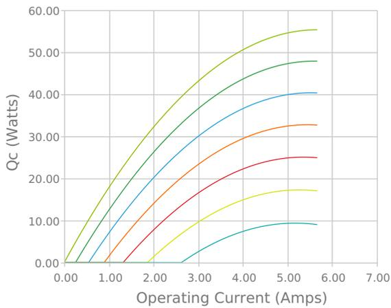
Heat Pumped at Cold Side
