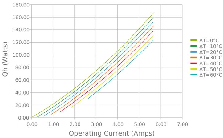
Total Heat Dissipated at Hot Side (Qh=Qc+Pin)
