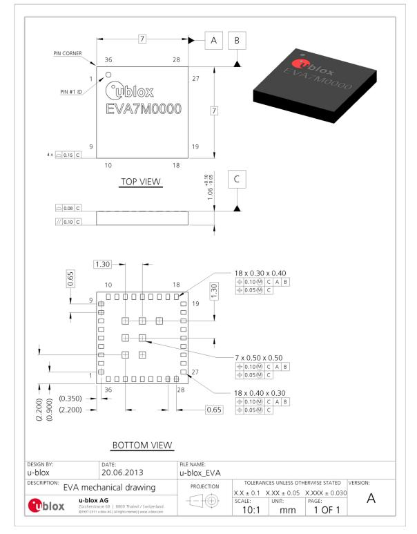
Figure 4: Mechanical drawing for EVA-7M (LGA43)
