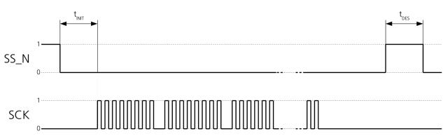
Figure 3: SPI timing diagram
