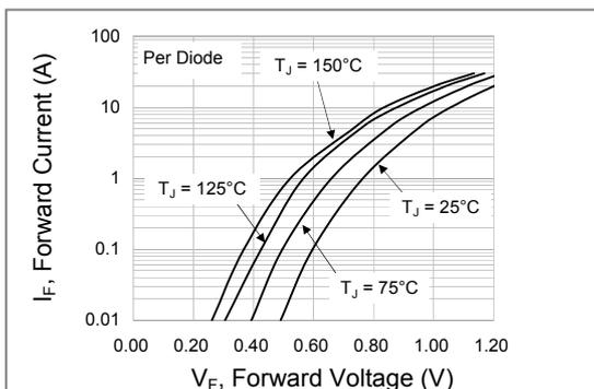
**Fig.7 UF2003FCT & UF2004FCT Typical Forward Characteristics**
