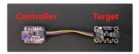
The I2C, or <u>inter-integrated circuit</u> (), is a 2-wire protocol for communicating with simple sensors and devices, which means it uses two connections, or wires, for transmitting and receiving data. One connection is a clock, called SCL. The other is the data line, called SDA. Each pair of clock and data pins are referred to as a bus.
