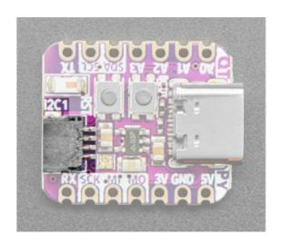
This JST SH 4-pin STEMMA QT () connector breaks out a second I2C interface (SCL1, SDA1, 3.3V, GND). It allows you to connect to various breakouts and sensors with STEMMA QT connectors () or to other things using assorted associated accessories (). It works great with any STEMMA QT or Qwiic sensor/device. You can also use it with Grove I2C devices thanks to this handy cable ().
