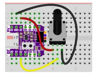
QT Py 3V to potentiometer left pin QT Py A2 to potentiometer middle pin QT Py GND to potentiometer right pin
