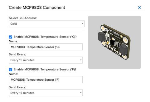
The MCP9808 sensor can measure ambient temperature. This page has individual options for reading the ambient temperature, in either Celsius or Fahrenheit. You may select the readings which are appropriate to your application and region.
