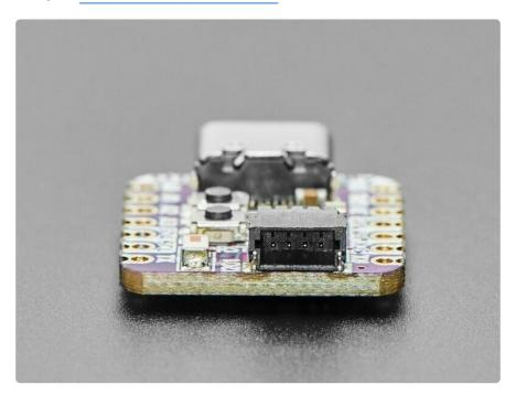
Pinout and shape are <u>Seeed Xiao</u> () compatible, with castellated pads. In addition to the QT connector, we also added an RGB NeoPixel (with controllable power pin to allow for ultra-low-power usage), a reset button (great for restarting your program or entering the bootloader) and a button on GPIO 0 for entering the ROM bootloader or for user input
