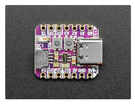
The ESP32-S2 is a highly-integrated, low-power, 2.4 GHz Wi-Fi System-on-Chip (SoC) solution that now has built-in native USB as well as some other interesting new
