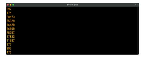
What do these values mean? In CircuitPython ADC values are put into the range of 16-bit unsigned values. This means the possible values you'll read from the ADC fall within the range of 0 to 65535 (or 2^16 - 1). When you twist the potentiometer knob to be near ground, or as far to the left as possible, you see a value close to zero.
