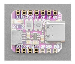
There are eleven GPIO pins broken out to pads. There is hardware I2C, UART, and SPI.
