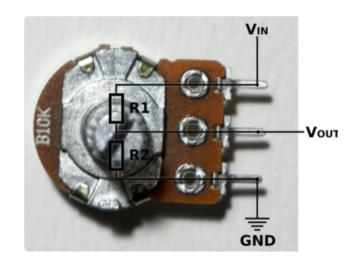
Connect one outside pin to ground Connect the other outside pin to voltage in (e.g. 3.3V) Connect the middle pin to an analog pin (e.g. A0)
