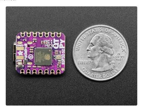
Please note the QT Py ESP32-S2 has a single-core 240 MHz chip, so it won't be as fast as ESP32's with dual-core. Also, there is no Bluetooth support. However, we are super excited about the ESP32-S2's native USB which unlocks a lot of capabilities for advanced interfacing! This ESP32-S2 mini-module we are using on the QT Py comes with 4 MB flash and 2 MB PSRAM so you can buffer massive JSON files for parsing!
