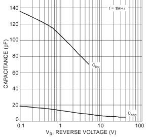
Fig. 6 Typical Capacitance Characteristics
