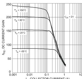
$\rm I_{C}$ , COLLECTOR CURRENT (A) Fig. 2 Typical DC Current Gain vs. Collector Current
