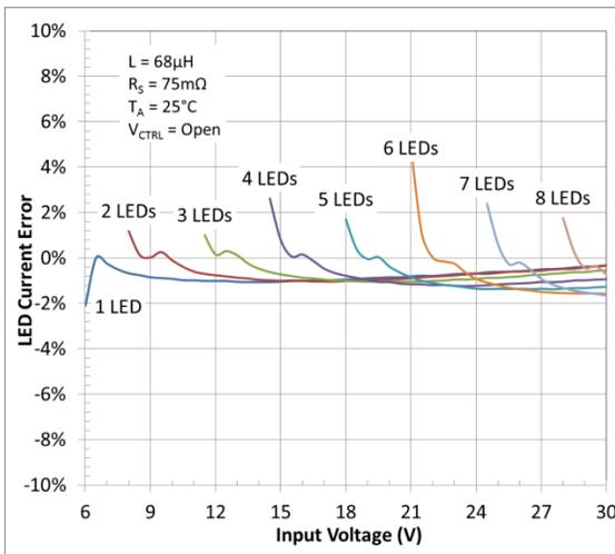
Figure 27. LED Current Deviation vs. Input Voltage
