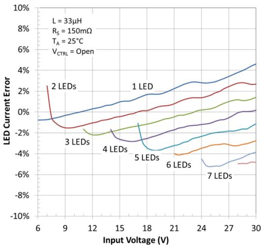
Figure 17. LED Current Deviation vs. Input Voltage
