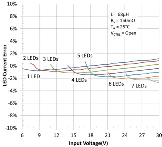
Figure 15. LED Current Deviation vs. Input Voltage
