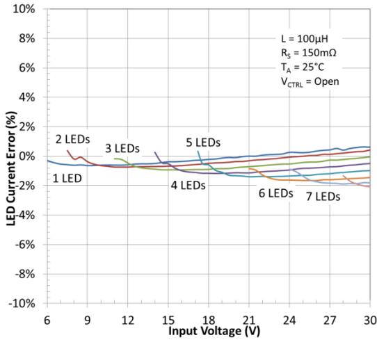
Figure 13. LED Current Deviation vs. Input Voltage
