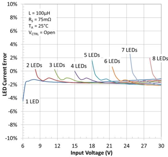
Figure 25. LED Current Deviation vs. Input Voltage
