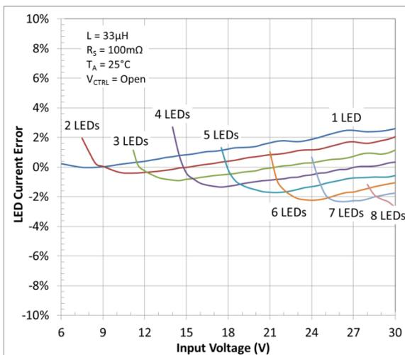
Figure 23. LED Current Deviation vs. Input Voltage
