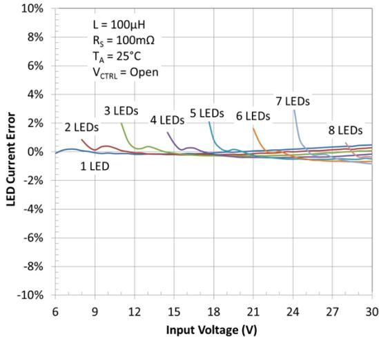
Figure 19. LED Current Deviation vs. Input Voltage
