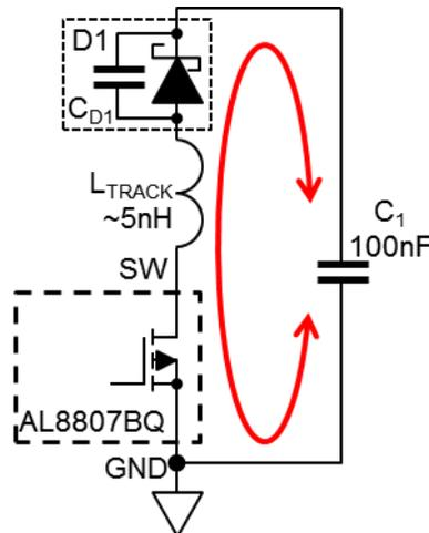
Figure 41 PCB Loop Resonance
