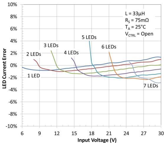
Figure 29. LED Current Deviation vs. Input Voltage
