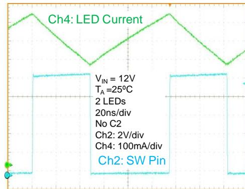
Figure 32 Typical Operating Waveform (C2 not fitted)
