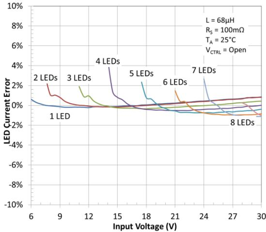
Figure 21. LED Current Deviation vs. Input Voltage
