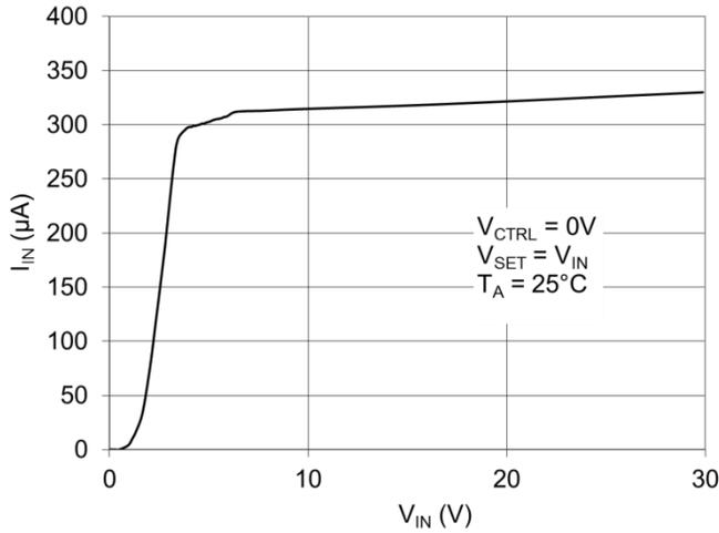
Figure 1. Supply Current (notswitching vs. Input Voltage)
