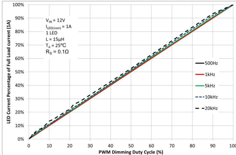
Figure 35 PWM Dimming at 530kHz nominal switching frequency
