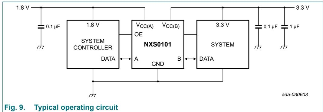
Fig. 9. Typical operating circuit
