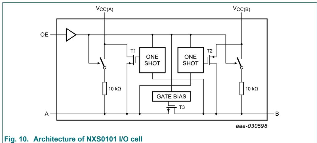
Fig. 10. Architecture of NXS0101 I/O cell
