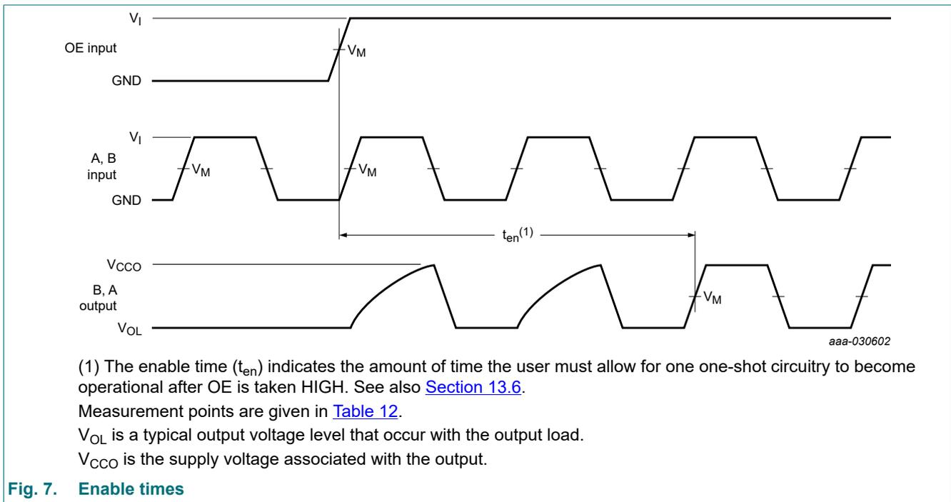
Fig. 7. Enable times
