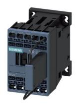
traction contactor, AC-3 12 A,  $5.5\,kW$  / 400 V 110 V DC, 0.7-1.25\*US with integrated suppressor diode 3-pole, size S00 spring-type terminal suitable for PLC outputs for upright mounting position not expandable with auxiliary switch
