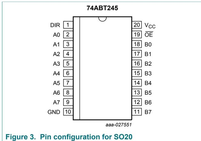
Figure 3. Pin configuration for SO20
