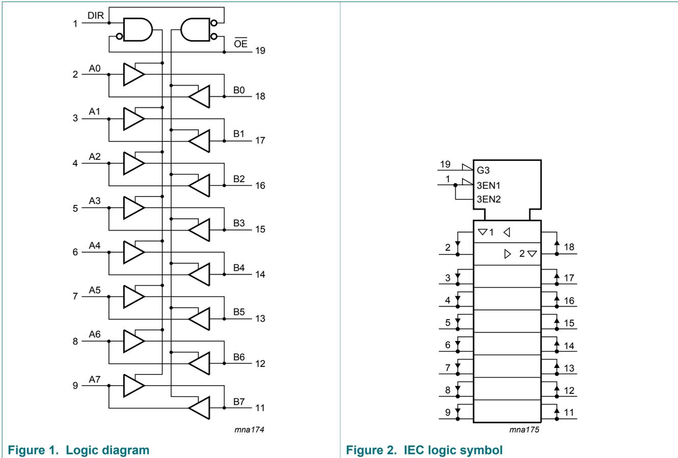
Figure 1. Logic diagram
