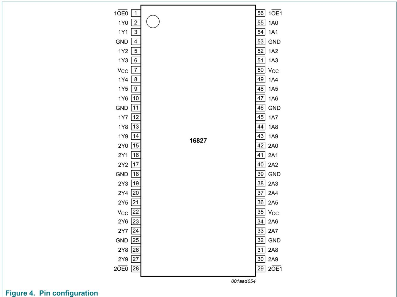
Figure 4. Pin configuration
