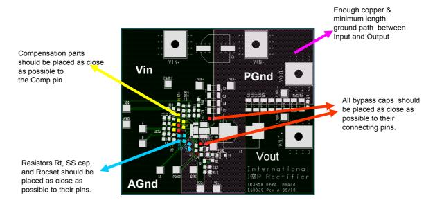
Fig. 28a. IRDC3856 demoboard layout considerations – Top Layer
