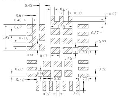
Stencil pad sizing (all dimensions in mm)
