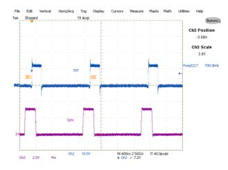
Fig. 26: Synchronization to 700kHz external clock signal at 6A load Ch<sub>2</sub>: SW (Switch Node) Ch<sub>3</sub>:Sync
