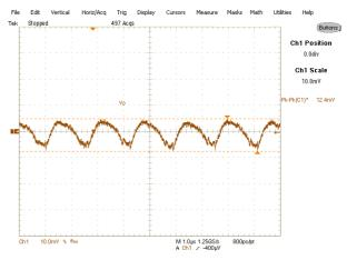
Fig. 21: Output Voltage Ripple, 6A load Ch<sub>1</sub>: V<sub>out</sub>
