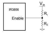
For a maximum Enable threshold of  $V_{EN}$  = 1.36 V
