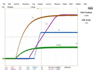
Fig. 18: Start up at 6A Load  $\mathrm{Ch_{1}:V_{in},\,Ch_{2}:V_{out},\,Ch_{3}:V_{ss},\,Ch_{4}:Enable}$
