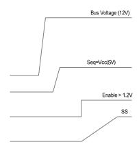
Fig. 3b. Recommended startup sequence, Non-Sequenced operation
