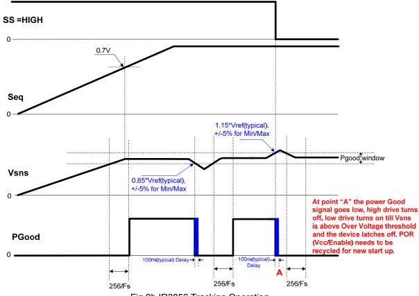
Fig.9b IR3856 Tracking Operation
