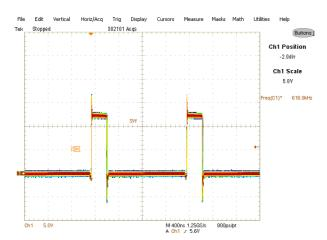
Fig. 22: Inductor node at 6A load Ch₁: Switch Node
