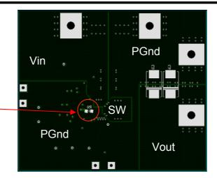
Single point connection between AGND & PGND; It — should be close to the SupIRBuck, kept away from noise sources.
