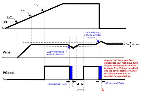
Fig.9a IR3856 Non-Tracking Operation (Seq=Vcc)
