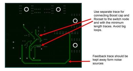
Fig. 28d. IRDC3856 demoboard layout considerations – Mid Layer 2
