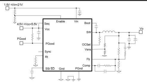
Fig. 1. Typical application diagram
