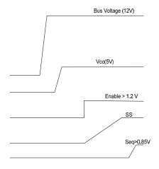
Fig. 3c. Recommended startup sequence, Sequenced operation
