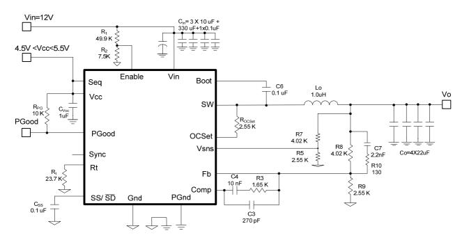
Fig. 17. Application circuit diagram for a 12V to 1.8 V, 6A Point Of Load Converter
