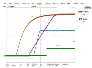
Fig. 19: Start up at 6A Load, Ch<sub>1</sub>:V<sub>in</sub>, Ch<sub>2</sub>:V<sub>out</sub>, Ch<sub>3</sub>:V<sub>ss</sub>, Ch<sub>4</sub>:V<sub>PGood</sub>
