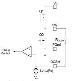
Fig. 7. Connection of over current sensing resistor
