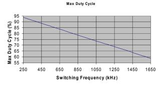
Fig. 11. Maximum duty cycle v/s switching frequency.
