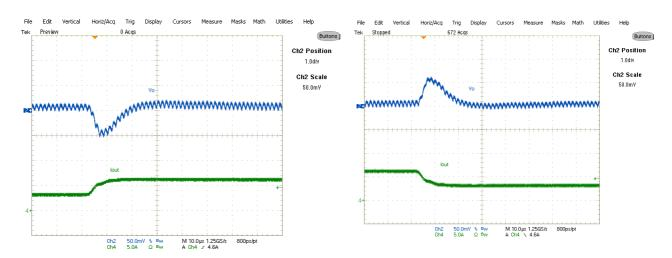
Fig. 24: Transient Response, 3A to 6A step  $2.5A/\mu s$   $Ch_2:V_{out}, Ch_4:I_{out}$
