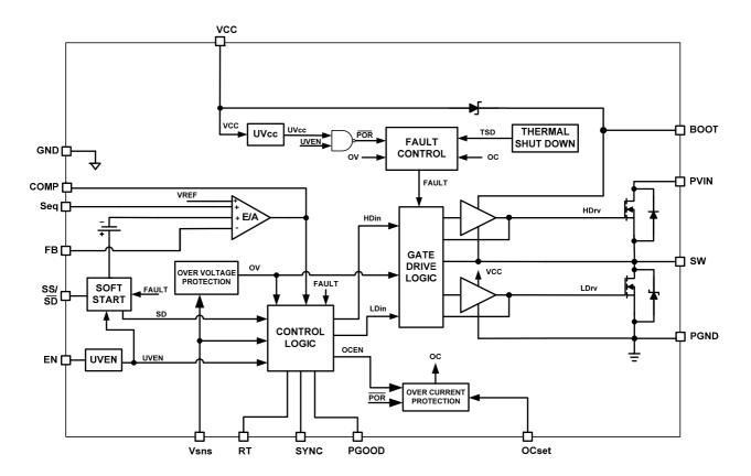
Fig. 2. Simplified block diagram of the IR3856
