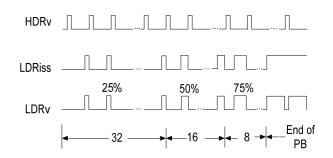
Fig. 5. Pre-Bias startup pulses
