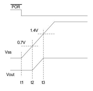
Fig. 6. Theoretical operation waveforms during soft-start
