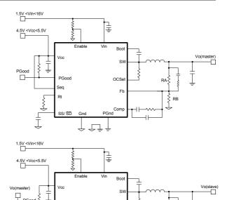
Fig. 8b. Application Circuit for Simultaneous Sequencing
