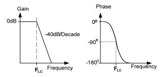
Fig. 14. Gain and Phase of LC filter
