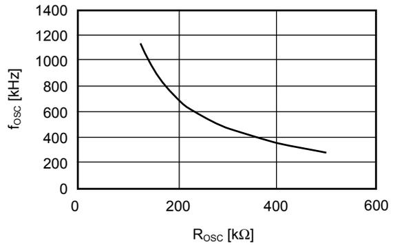
**Figure 12 R<sub>osc</sub> vs. f<sub>osc</sub>**
