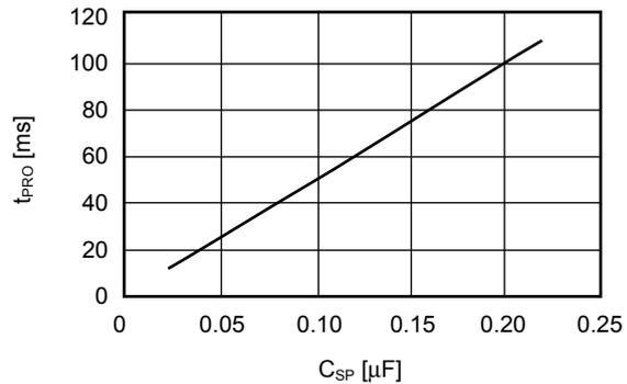
**Figure 14 C<sub>SP</sub> vs. t<sub>PRO</sub>**
