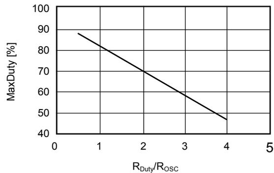
**Figure 13 R<sub>Duty</sub>/R<sub>osc</sub> vs. MaxDuty**
