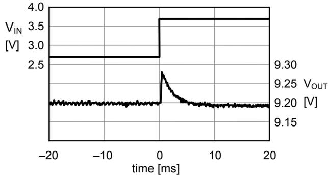
(2)  $f_{OSC} = 1133\text{ kHz}$ ,  $V_{IN} = 3.7\text{ V} \rightarrow 2.7\text{ V}$
