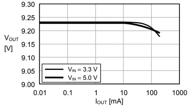
(2) f<sub>osc</sub> = 700 kHz, MaxDuty = 77 % (R<sub>osc</sub> = 200 kΩ, R<sub>Duty</sub> = 300 kΩ)
