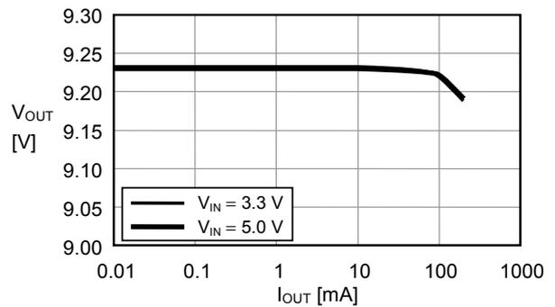
(3) f<sub>osc</sub> = 286 kHz, MaxDuty = 77 % (R<sub>osc</sub> = 510 kΩ, R<sub>Duty</sub> = 750 kΩ)
