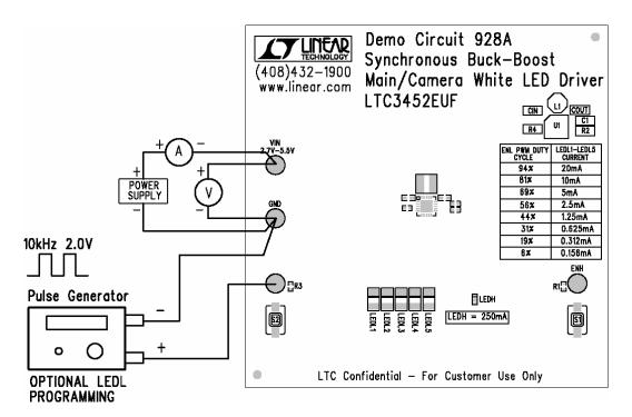
Figure 1. Proper Measurement Equipment Setup
