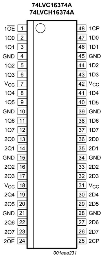
Fig. 5. Pin configuration SOT370-1 (SSOP48) and SOT362-1 (TSSOP48)
