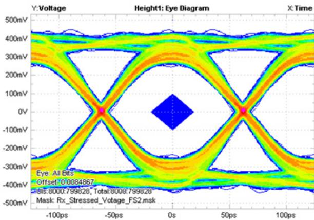
Figure 6. Reference PCIe 3.0 Eye Diagram without Switch at 8 Gbps, 800 mV<sub>pp</sub> Differential Swing
