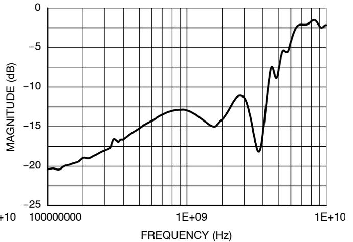
Figure 11. Differential Return Loss
