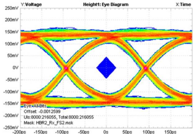
Figure 5. DisplayPort 1.2 Eye Diagram through NCN3612B at 5.4 Gbps, 340 mV<sub>pp</sub> Differential Swing
