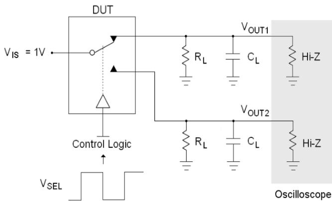
Figure 17.  $t_{ON}$  and  $t_{OFF}$
