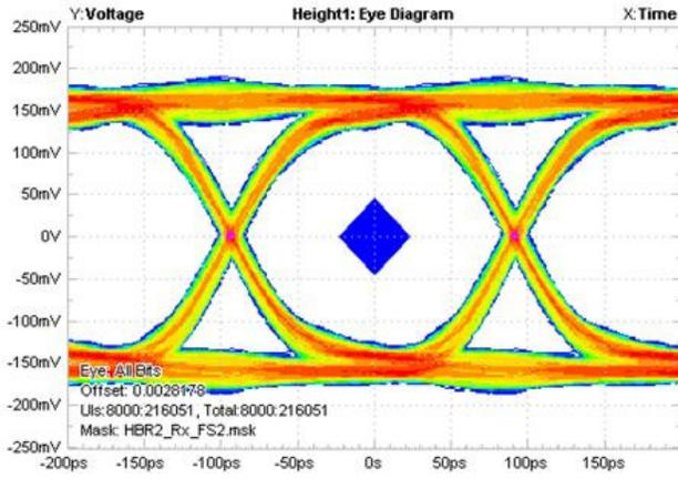
Figure 4. Reference DisplayPort 1.2 Eye Diagram without Switch at 5.4 Gbps, 340 mV<sub>pp</sub> Differential Swing
