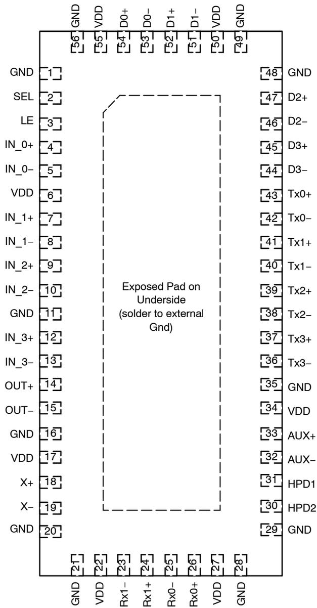
**Figure 3. Pinout
