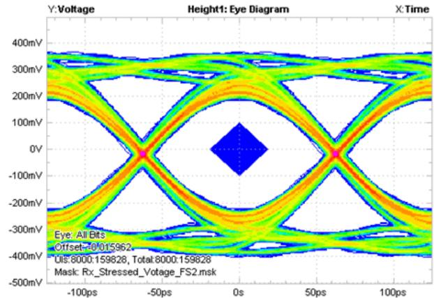
Figure 7. PCIe 3.0 Eye Diagram through NCN3612B at 8 Gbps, 800 mV<sub>pp</sub> Differential Swing
