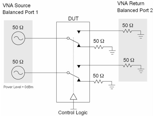
Figure 14. Differential Off Isolation ( $S_{DD21}$ )
