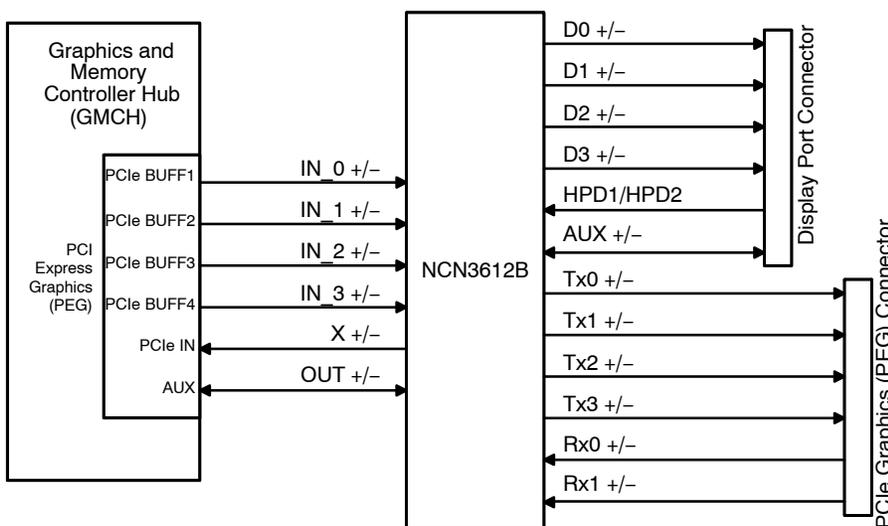
Figure 1. Application Schematic
