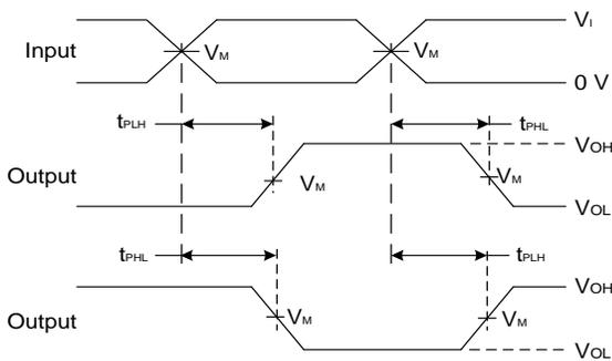
**Voltage Waveform Propagation Delay Times
