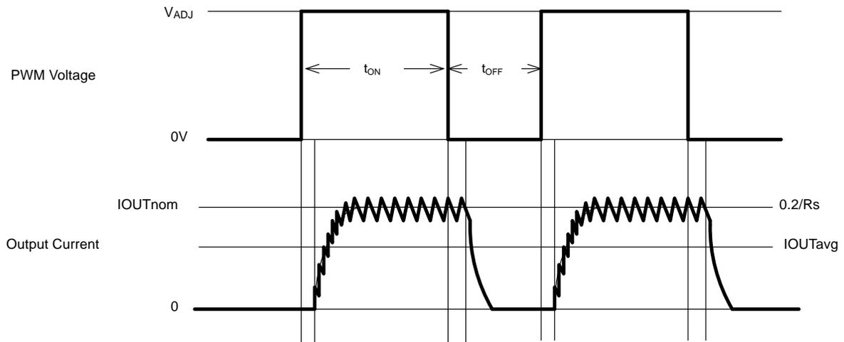
Figure 8. Low Frequency PWM Operating Waveforms
