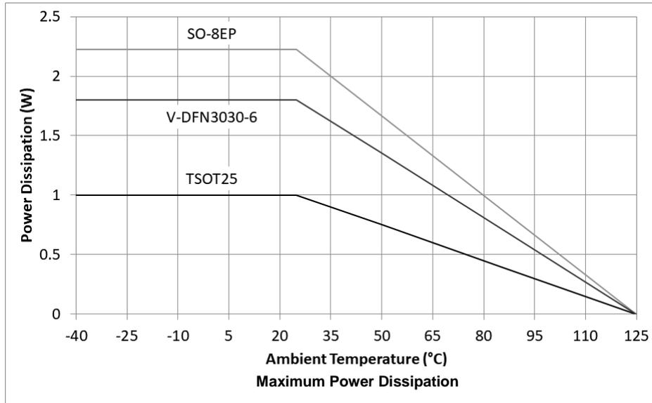
Note that the device power dissipation will most often be a maximum at minimum supply voltage. It will also increase if the efficiency of the circuit is low. This may result from the use of unsuitable coils, or excessive parasitic output capacitance on the switch output.
