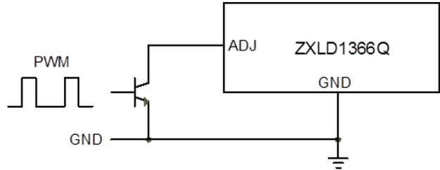
This scheme uses the 50k resistor between the ADJ pin and the internal voltage reference as a pull-up resistor for the external transistor.
