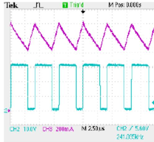
$V_{IN} = 60V$ ,  $R_S = 0.2\Omega$ ,  $L = 68\mu H$  Normal Operation.
