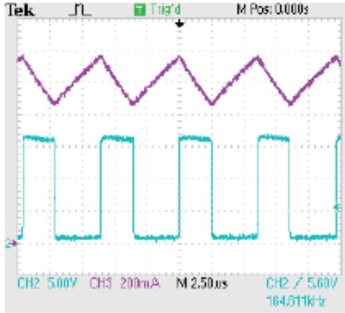
$V_{IN} = 30V$ ,  $R_S = 0.2\Omega$ ,  $L = 68\mu H$  Normal Operation.
