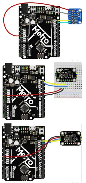
Connect Vin to the power supply, 3-5V is fine. Use the same voltage that the microcontroller logic is based off of. For most Arduinos, that is 5V (red wire on STEMMA)
