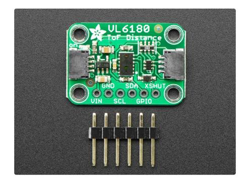
The sensor is small and easy to use in any robotics or interactive project. Since it needs 2.8V power and logic we put the little fellow on a breakout board with a regulator and level shifting. You can use it with any 3-5V power or logic microcontroller with no worries. Each order comes with a small piece of header. Solder the header onto your breakout board with your iron and some solder and wire it up for instant distance-sensing-success!
