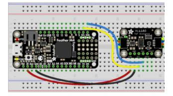
Board GND to sensor GND (black wire) Board 3V to sensor VIN (red wire) Board SDA to sensor SDA (blue wire) Board SCL to sensor SCL (yellow wire)
