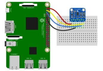
Pi 3V3 to sensor VIN Pi GND to sensor GND Pi SCL to sensor SCL Pi SDA to sensor SDA
