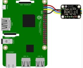
Here's the Raspberry Pi wired with I2C:
