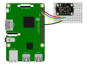
Pi GND to sensor GND (black wire) Pi 3V3 to sensor VIN (red wire) Pi SDA to sensor SDA (blue wire) Pi SCL to sensor SCL (yellow wire)
