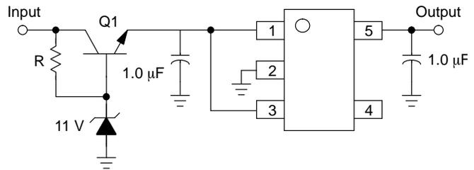
**Figure 24. Input Voltages Greater than 12 V**
