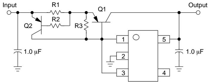
**Figure 22. Current Boost Regulator with Short Circuit Limit**
