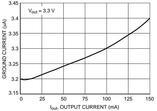
**Figure 3. Ground Pin Current versus Output Current**
