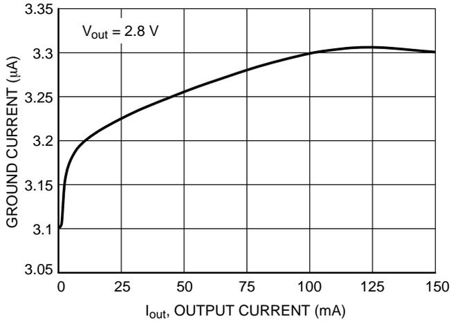
**Figure 2. Ground Pin Current versus Output Current**
