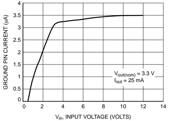
**Figure 5. Ground Pin Current versus Input Voltage**
