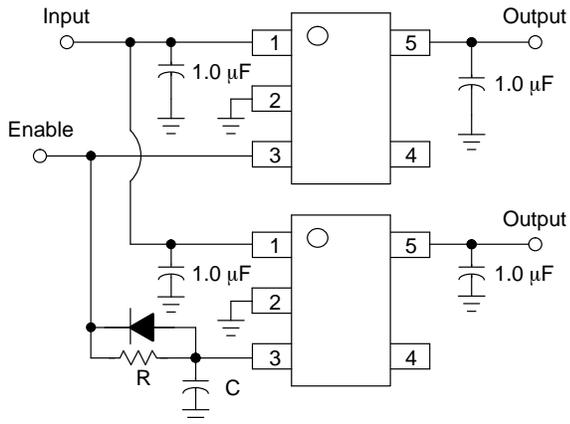
**Figure 23. Delayed Turn-on**
